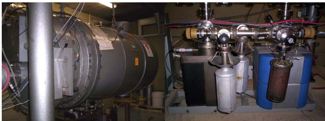
Fig. 16 System of vacuum pumps (left). Pressurized tank, where, in the atmosphere of inert gas, the accelerating column is placed (right)
