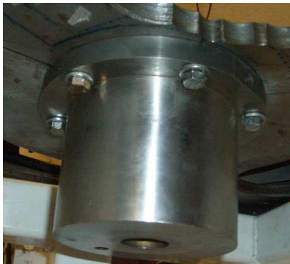
Fig. 37 Metal block bolted to housing base
