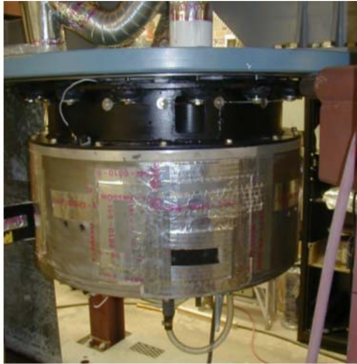
Fig. 49 Test rig bolted to spin pit flange
