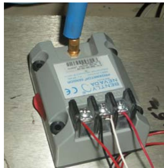
Fig. 44 Proximator for speed sensor connection
