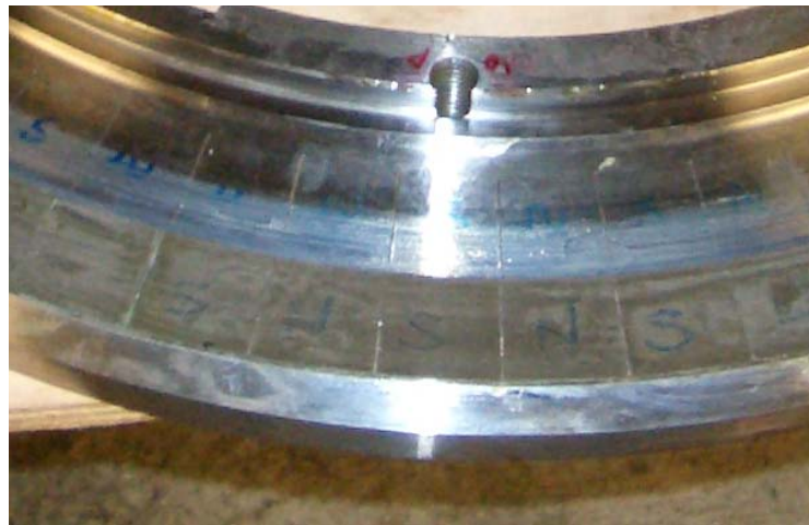
Fig. 7 North-South array magnet arrangement
