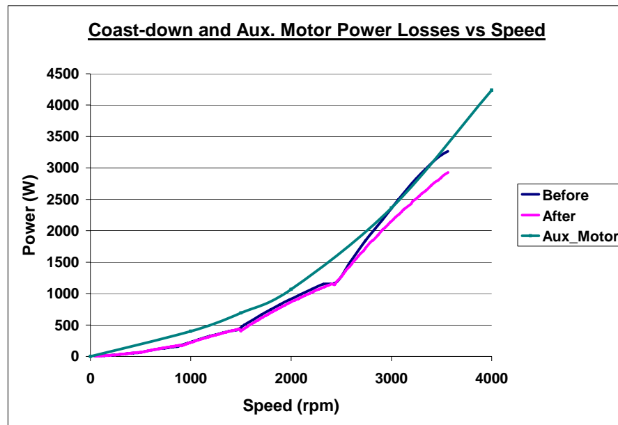
Fig. 88 Power loss comparison between coast down and auxiliary motor
