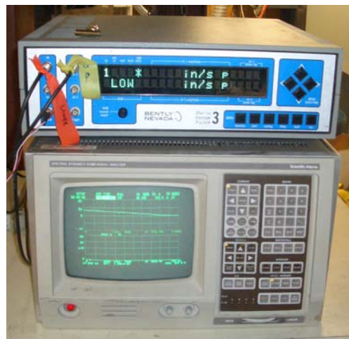
Fig. 46 Digital vector filter (top) and oscilloscope (bottom)
