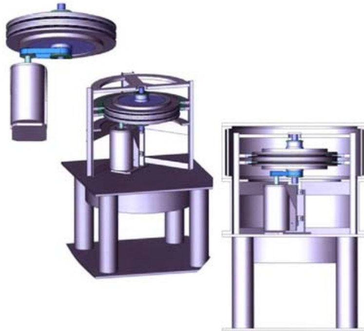
Fig. 2 Test motor coupled with auxiliary motor [6]
