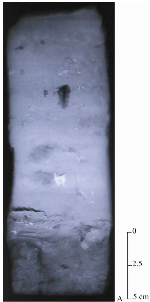
Figure 6: X-radiograph from a core from the Redfish Island survey area showing the no stratification and intermittent oyster shell debris. The black area in the center of the image is an anomaly caused by an air bubble trapped between the core and the x-ray tray.
