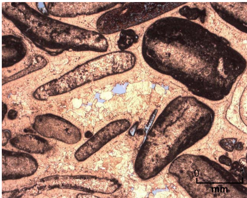
Figure B-6. Thin section photo from Jade #1 @ 6,799' Pore types CRIC, M, and SEIP Phylloid Algal Fragments
