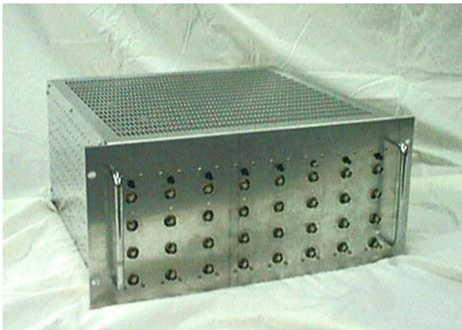
Fig. 51. A 19-in. chassis containing one of the two, 32-channel RF to IF conversion modules.
