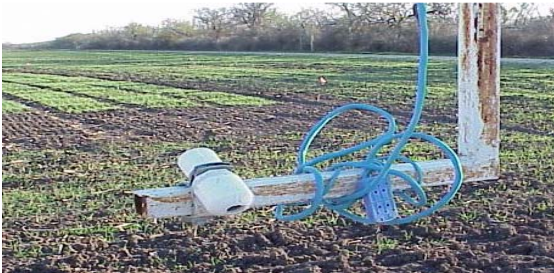
Fig. 2. Pivot-mounted IRTs. The IRTs were used to scan cotton canopy temperatures as the pivot was moving across the field. The IRTs are positioned at 15-foot spacings with a 1:1 meter height to view angle ratio.
