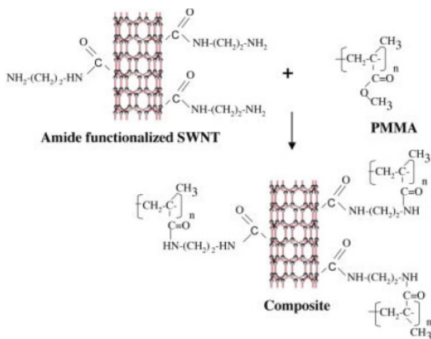
Figure 1.20 Amide covalent functionalization of SWNTs used to improve dispersion of SWNT-PMMA composite 104
