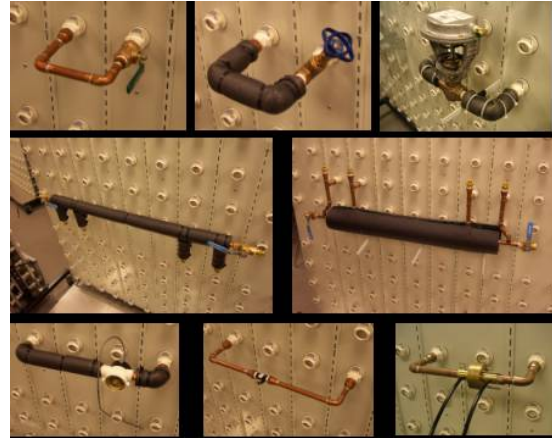
Figure 1. A variety of breadboard compatible valve (butterfly, globe, and pneumatically actuated), heat exchanger (single and multiple pass), and flow sensor (paddlewheel, turbine, and orifice plate) assemblies.
