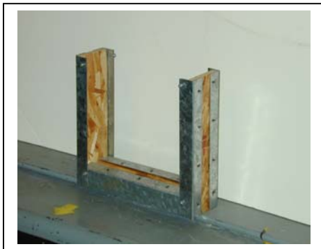
Figure 3. FSEC steel/ wood stud.
