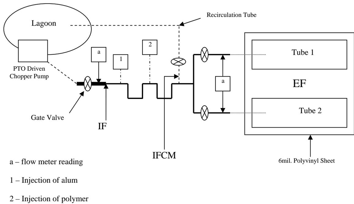
Figure 7. Schematic of the Geotube<sup>®</sup> dewatering system components (not to scale)
