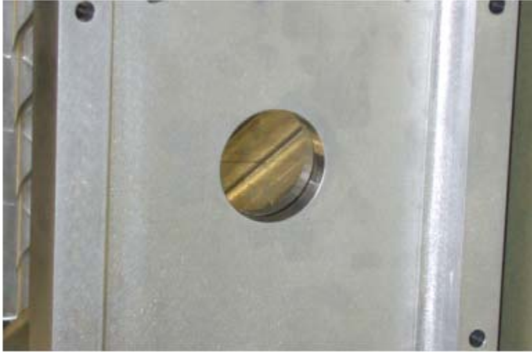
Figure A.16 Two-Inch Diameter Wiring Hole
