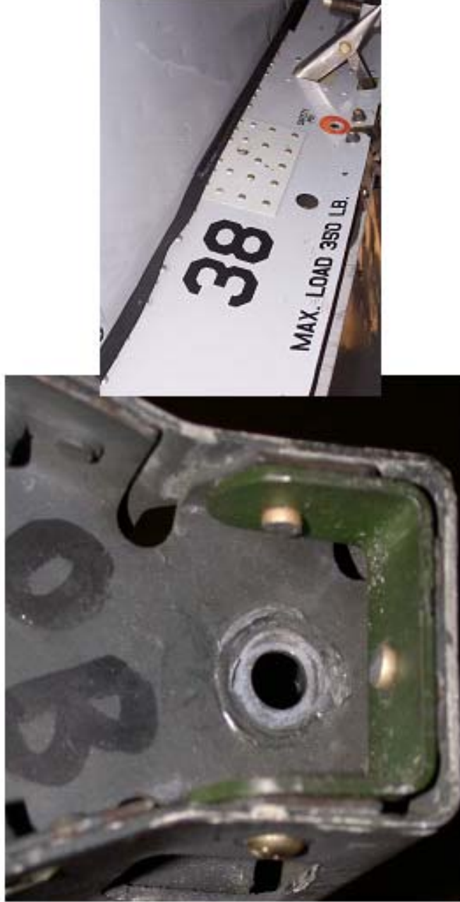
Figure A.42 Stiffeners Applied to Pylon Skin
