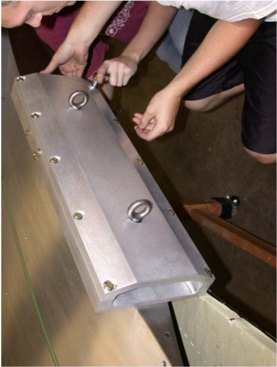
Figure A.10 Airfoil Mounting Structure
