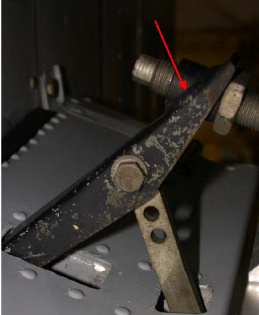
Figure A.37 Weld on Original Rocker Arm Assembly
