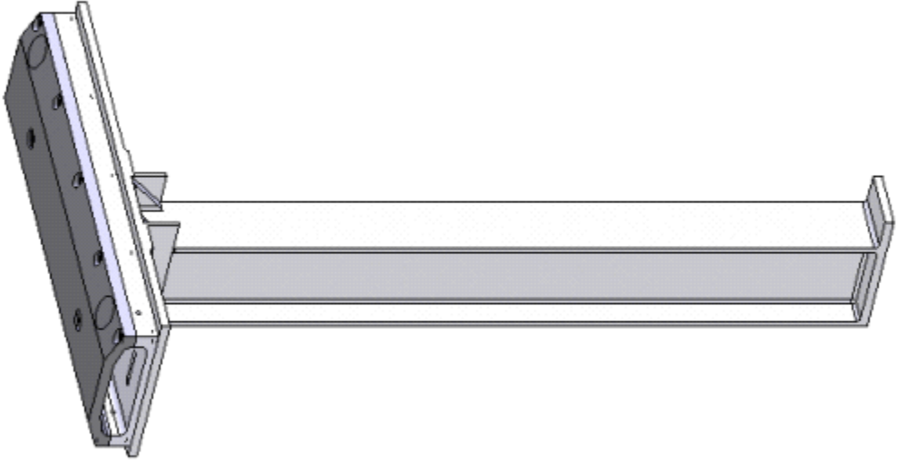
Figure A.51 Static Model Used to Simulate True Airfoil Model
