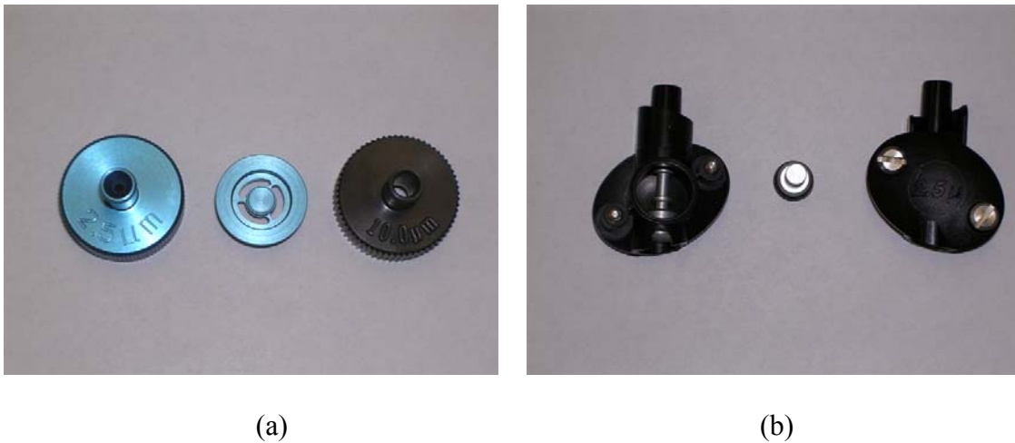
FIGURE 2-9. Impactors used as size selective pre-filters in real-time monitors.
