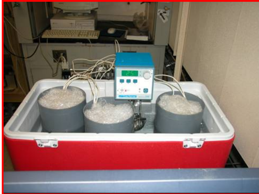
Fig. 28. Temperature-Controlled System (Temperature Regulator, Water in Ice Chest, and Plastic Mold)
