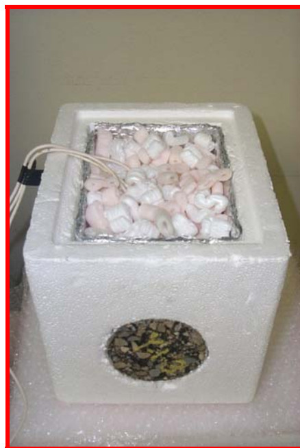
Fig. 26. HMA Specimen with One Uncovered Surface Covered with Packing Foam Material
