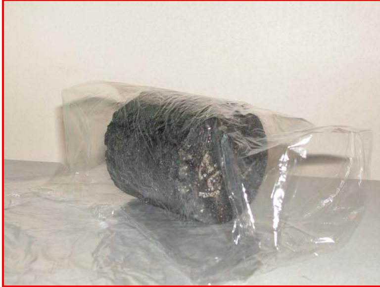
Fig. 56. Specimen Wrapped with Plastic Wrap
