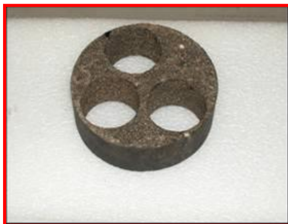
Fig. 65. Gyrotory Specimen after Coring of Test Specimens
