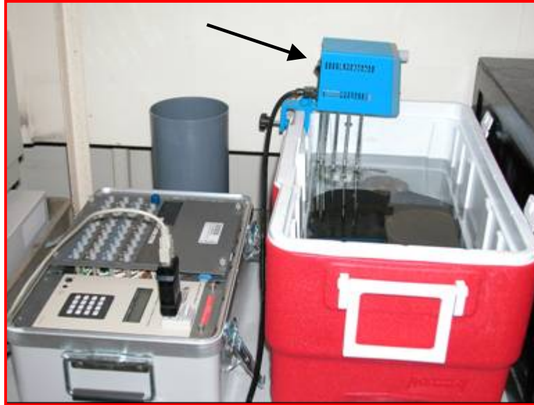
Fig. 14. Temperature Controller to Maintain Temperature during Calibration
