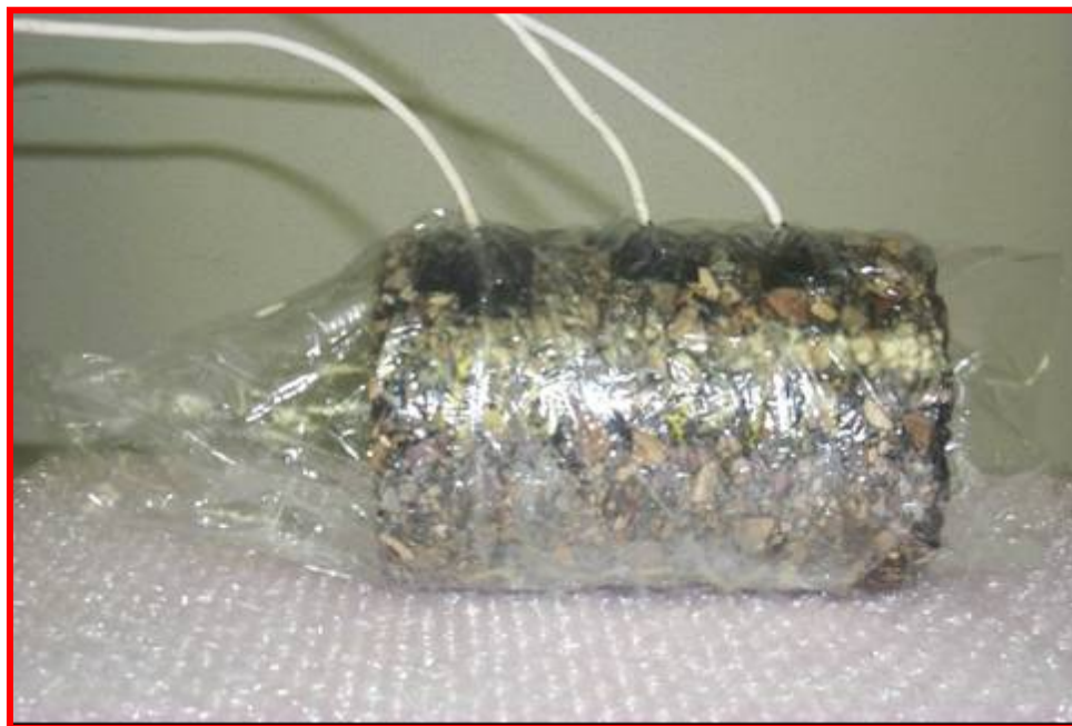
Fig. 22. Wrapping HMA Specimen with Two Layers of Plastic Clear Wrap
