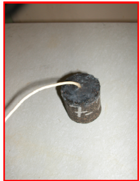
Fig. 70. Sealing Hole and Covering Upper Side with Silicon Glue
