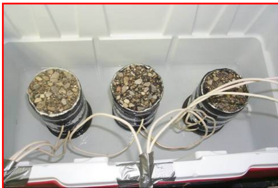
Fig. 24. Placing HMA Specimens in Bath of Water
