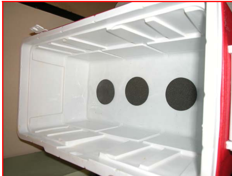
Fig. 59. Porous Stones Placed in Bath of Water
