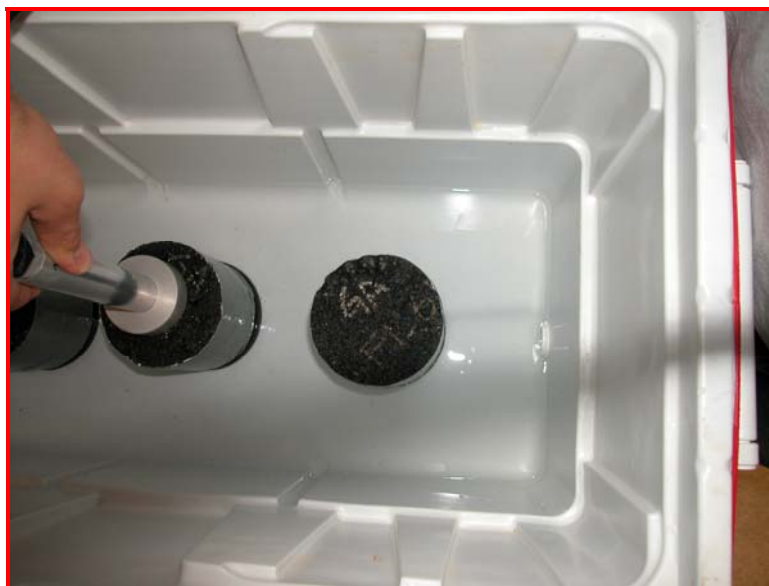
Fig. 61. Percometer Used to Record Dielectric Values
