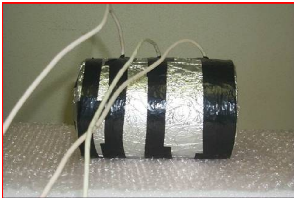
Fig. 23. Wrapping HMA Specimen with Aluminum Foil and Supported with Plastic Tape
