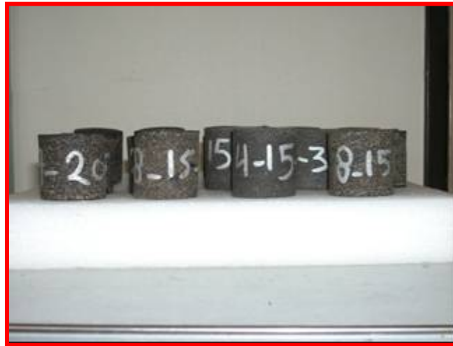
Fig. 66. Sand Asphalt Specimens after Coring Gyrotory Compacted Mixes
