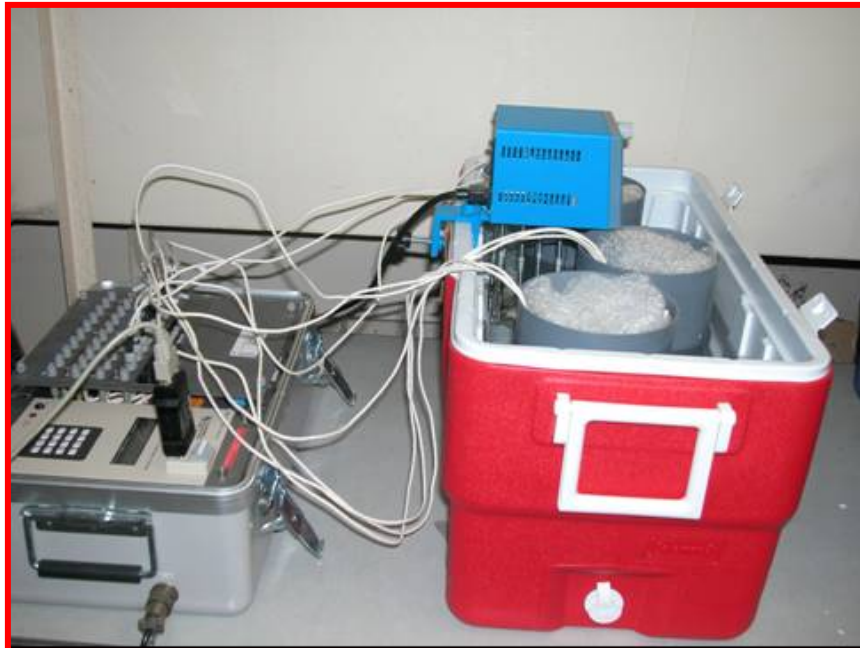
Fig. 30. Psychrometers Connected to CR-7 Datalogger
