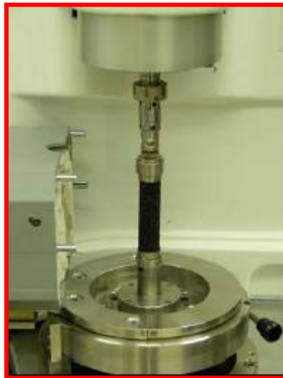
Fig. 73. Asphalt Sand Specimen Mounted in DMA (Zollinger 2005)
