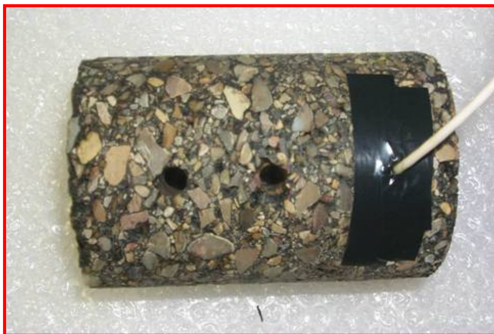
Fig. 20. Covering Holes with Plastic Tape
