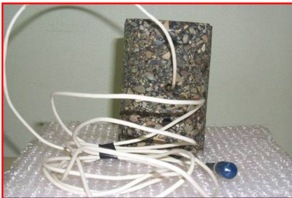
Fig. 18. Inserting Psychrometer in HMA Hole
