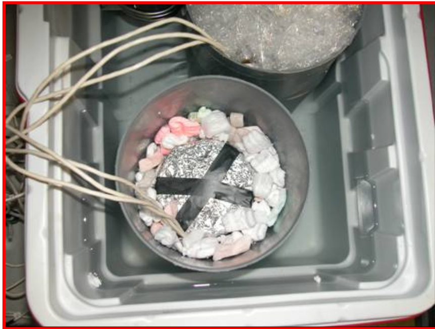
Fig. 27. HMA Specimen Placed in Plastic Mold
