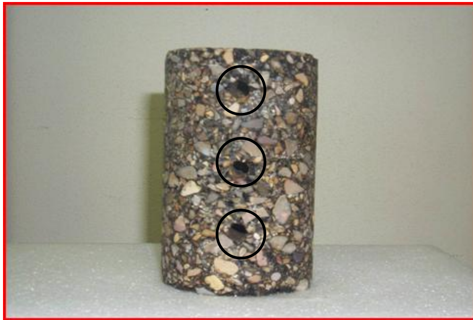
Fig. 17. HMA Specimen with Three Holes for Psychrometers
