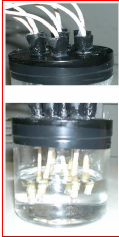
Fig. 13. Psychrometers Suspended in Calibration Solution (Sood 2005)
