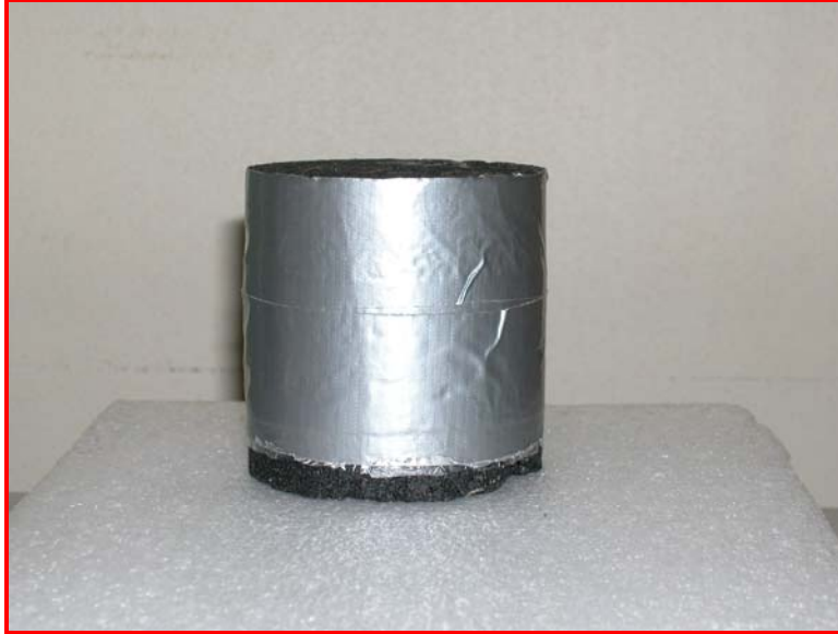
Fig. 58. Plastic Tape Is Used to Fasten the Wrap
