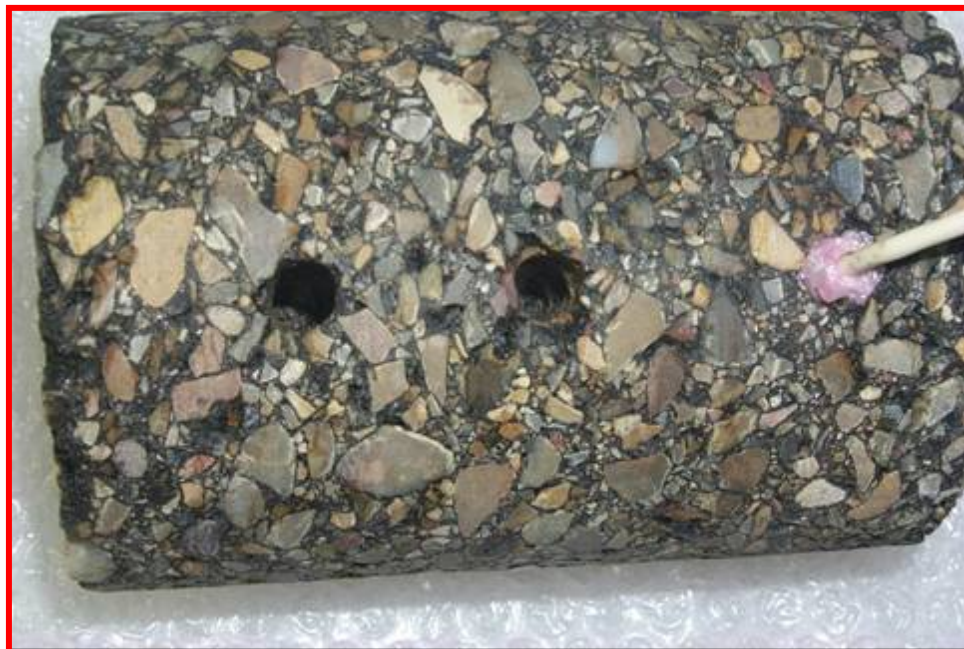
Fig. 19. Filling Holes with Filler
