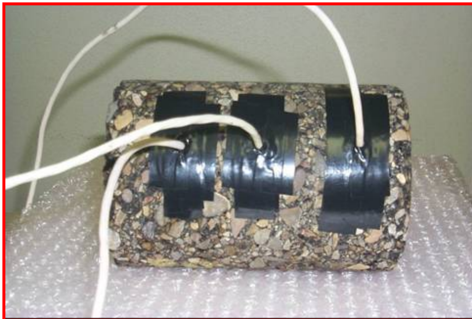
Fig. 21. Three Psychrometers Inserted in HMA Specimen
