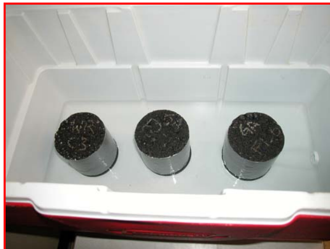
Fig. 60. HMA Mixes Placed over Porous Stones in Bath of Water
