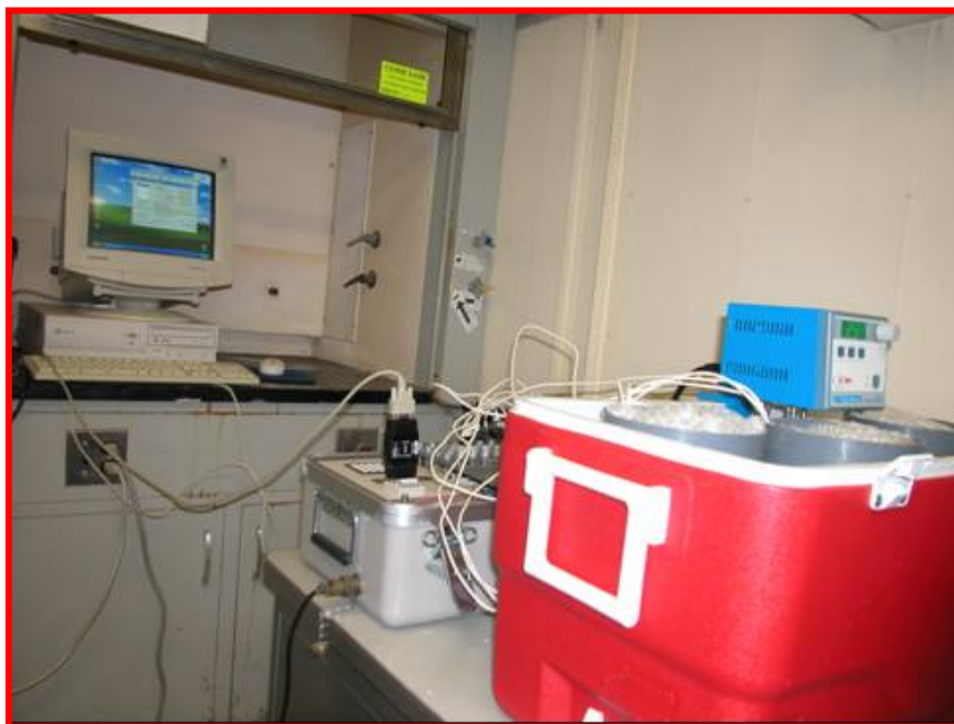
Fig. 31. Computer Connected to CR-7 Datalogger
