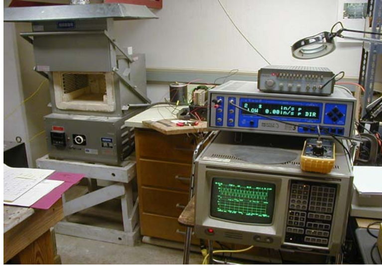
Figure 4.2 Actual Setup for testing magnetic properties of AISI 1010
