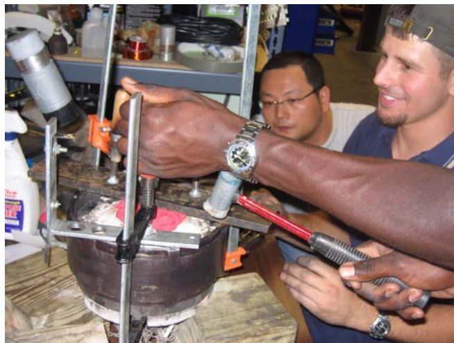
Figure 5.6 The Assembly Process of Stator in Back Iron with Special Tool
