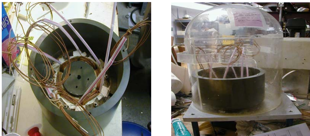
Figure 5.4 The Molding Process of the Bearing
