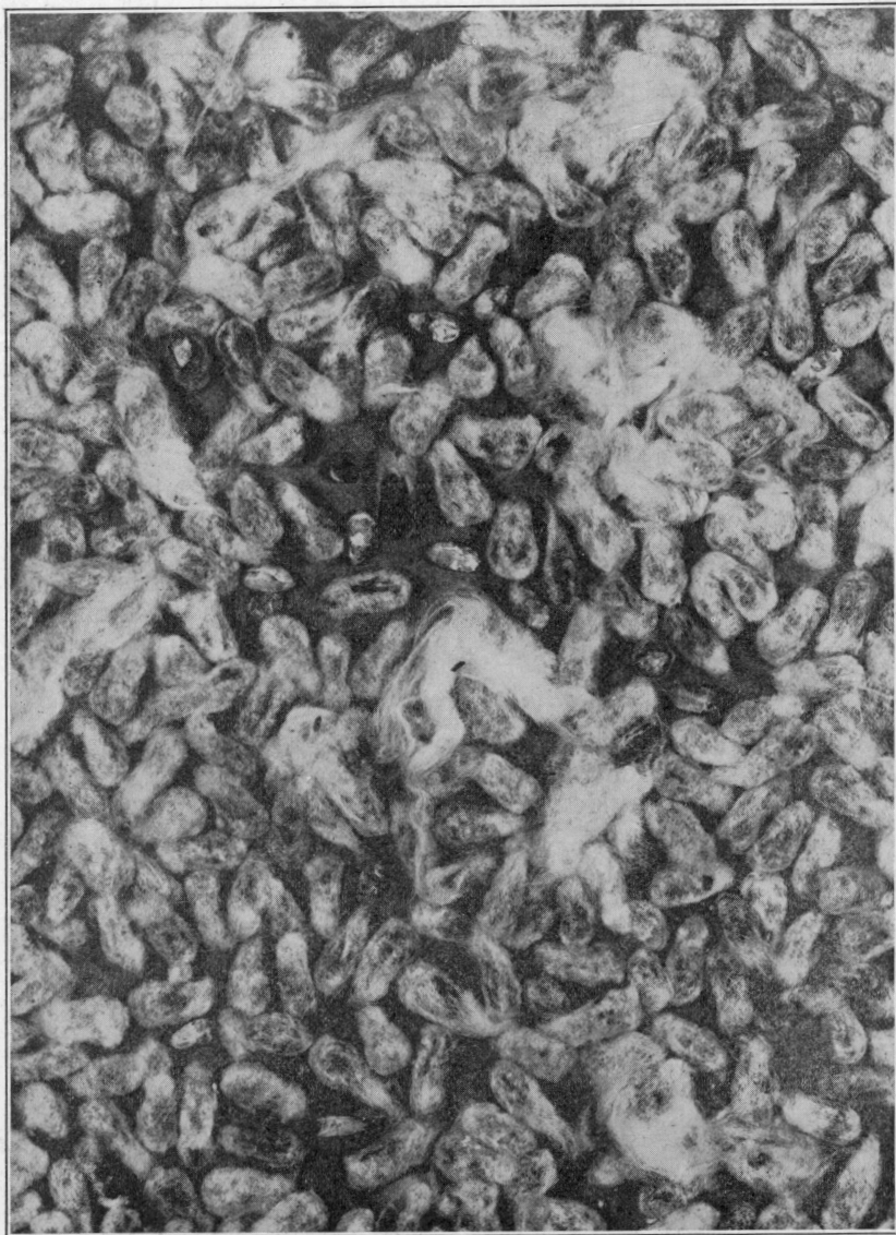
Figure 10.—Sample of seed ginned under poor conditions of ginning, which were a saw speed of 840 revolutions per minute, a tight breast-roll, and non-use of the standard air-line cleaner. Note that some of the seed are not well cleaned, while others are broken and hulled.
