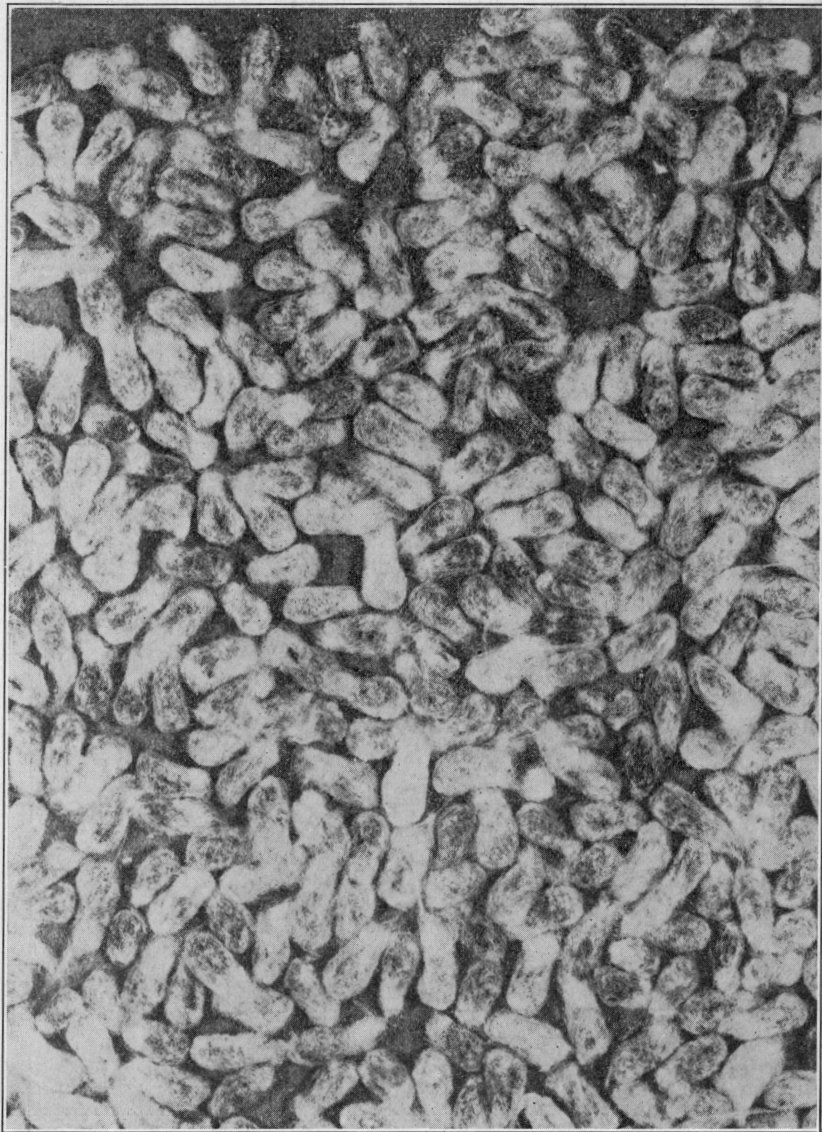
Figure 9.—Sample of seed ginned under good conditions of ginning, which were a saw speed of 760 revolutions per minute, a loose breast-roll, and the use of the standard air-line cleaner.
