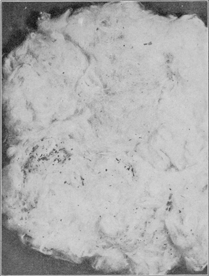
Figure 8.—Sample of lint cotton ginned under poor conditions of ginning, which were a saw speed of 840 revolutions per minute, a tight breast-roll, and non-use of the standard air-line cleaner. Note the presence of neps, gin-cuts, and trash.
