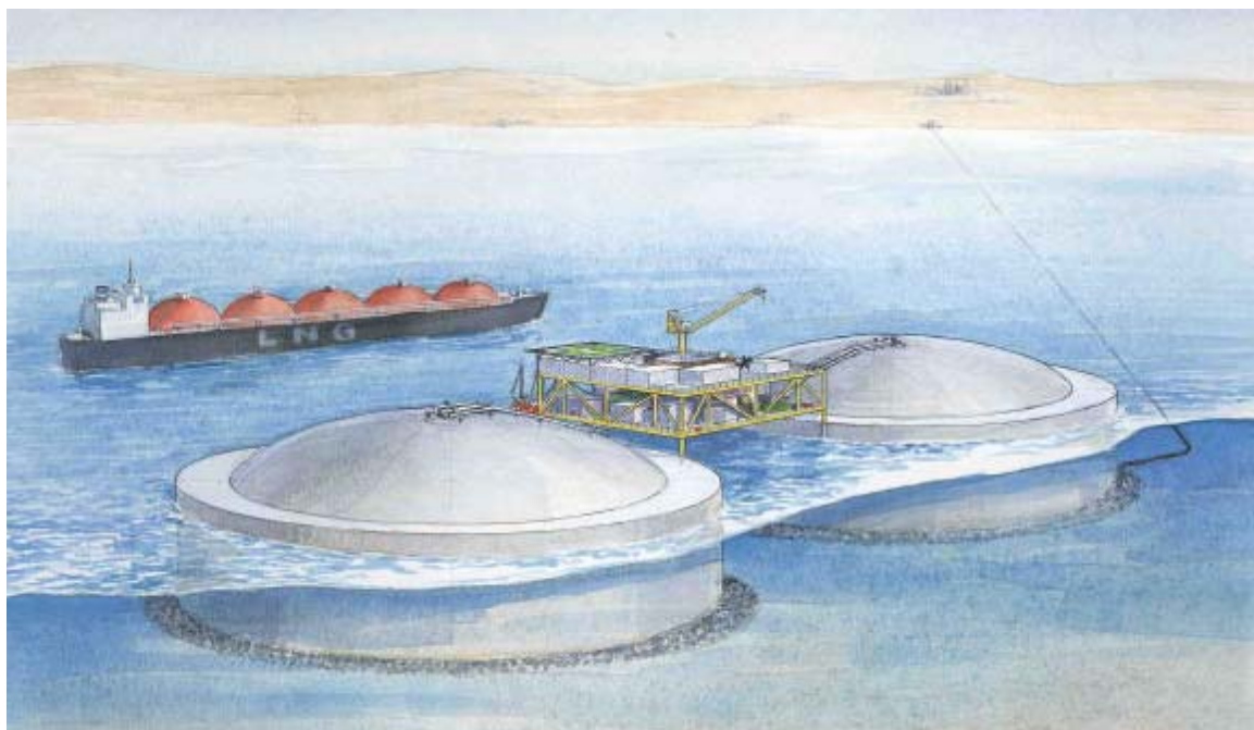
Fig. 11. A Novel Concept for Offshore LNG Storage Based on Primary Containment in Concrete
