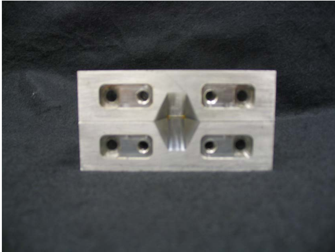
Figure 31. View of accelerator for second stage impactor.
