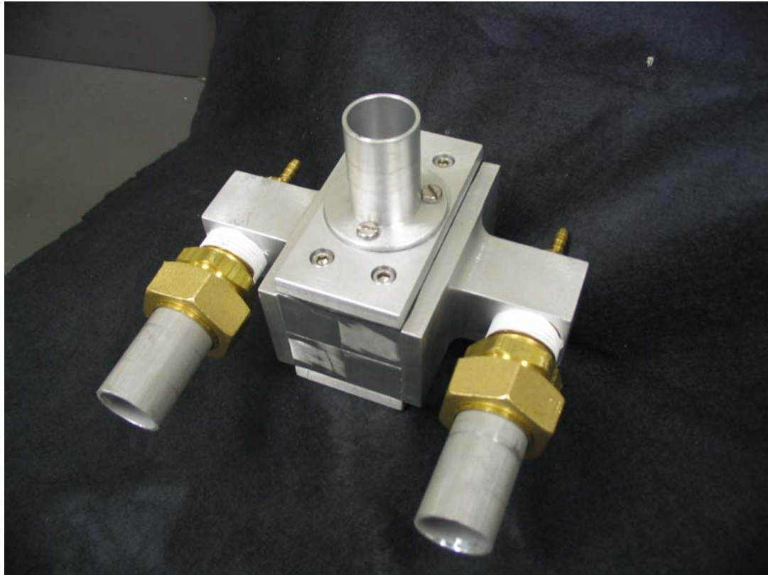
Figure 32. Aerosol transport fixtures for second stage impactor.
