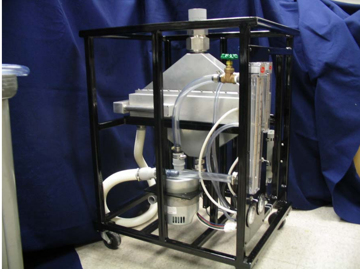
Figure 3. Breadboard system for multi-nozzle two-stage impactor.
