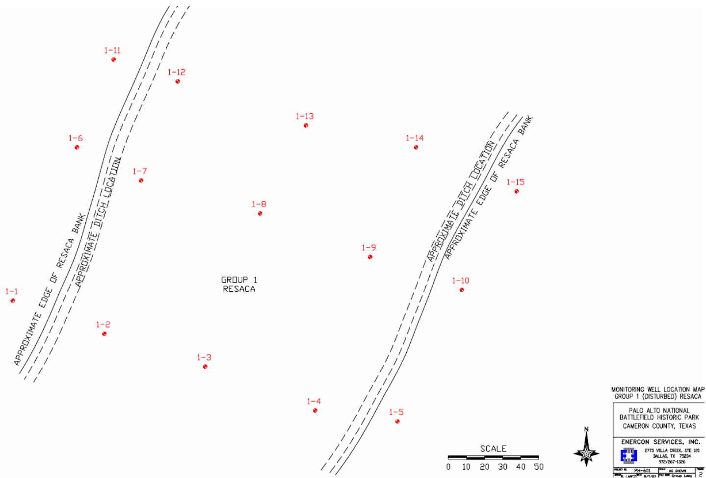
Fig. 3.3. Monitoring well location map for Group 1. A total of 15 wells were installed along three transects spanning the width of the disturbed resaca . Location map from Groundwater Monitoring Well Installation Report, Enercon Services, Inc. 2003.
