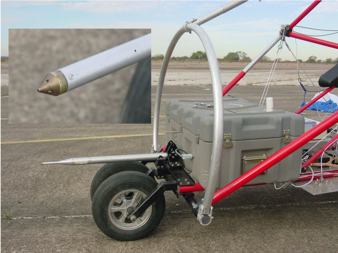
Figure 4.2 5-Hole Multifunction Aeroprobe Installed on Buckeye
