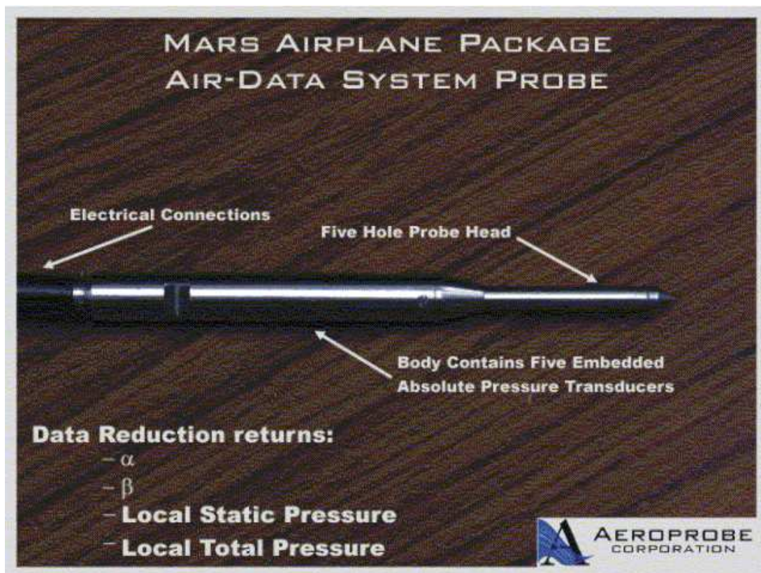
Figure 4.1 5-Hole Multifunction Aeroprobe, Courtesy of Aeroprobe Corp.
