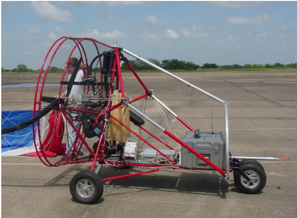
Figure 1.3 Modified Buckeye Test Bed
