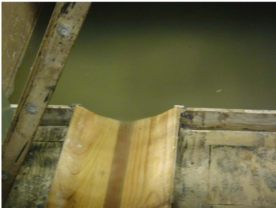
Figure B.20 Smooth flow transition at the exit of Flume Test 10
