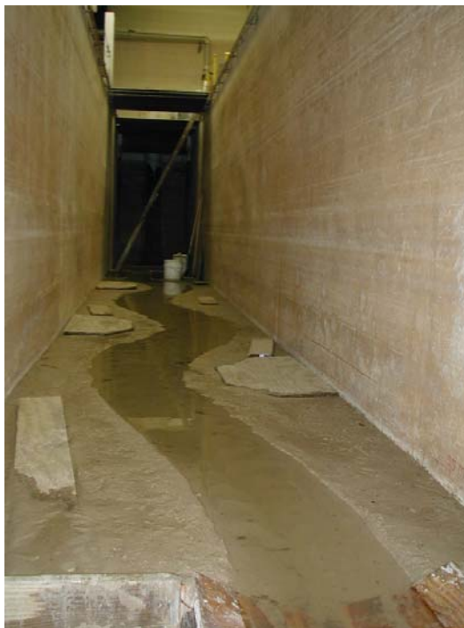
Figure B.24 Flume Test 13 is running, looking downstream
