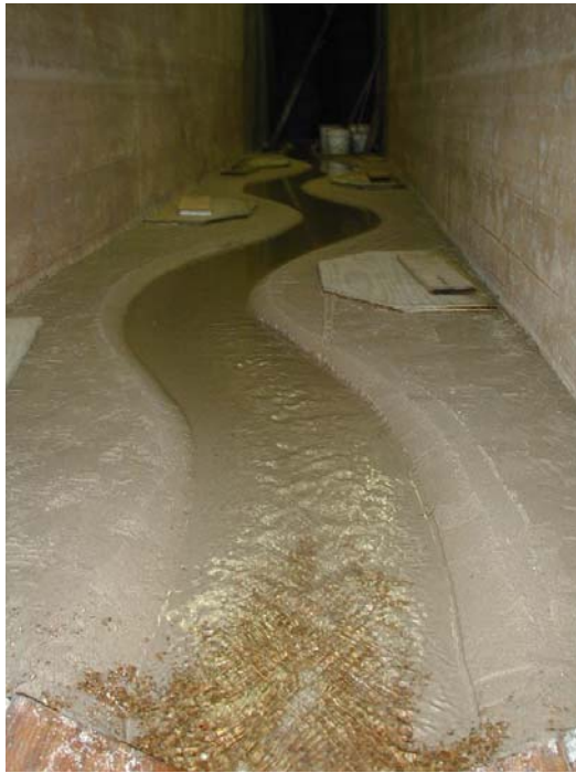
Figure B.21 Flume Test 11 with reinforcement at entry, looking downstream
