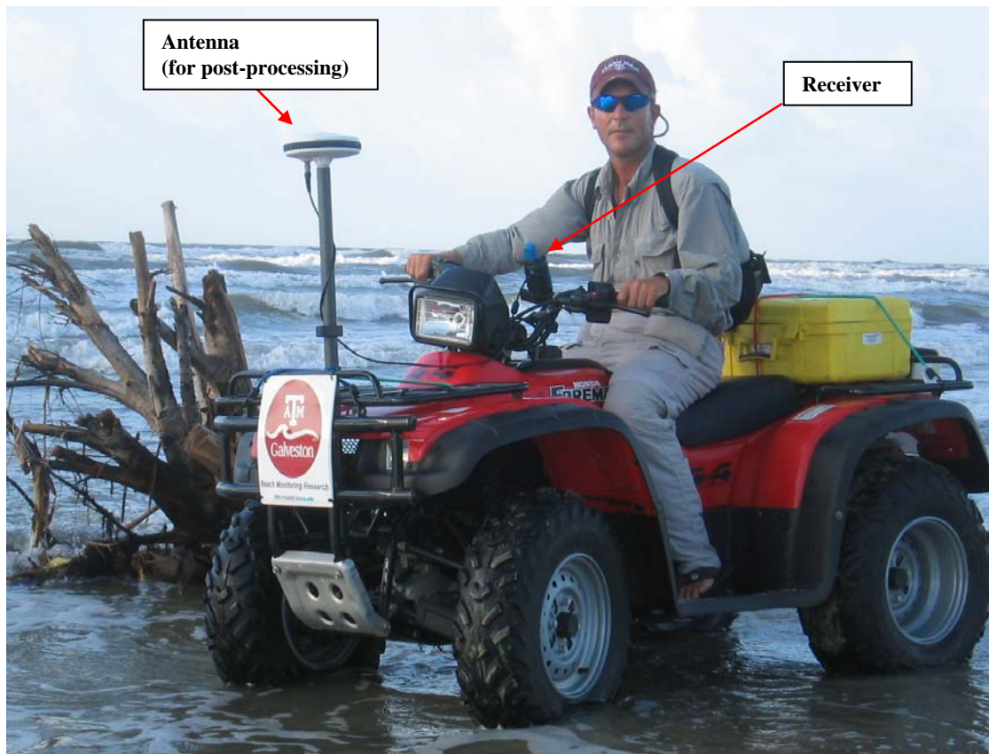
Figure 3. ATV mounted with post-processed differential kinematic GPS receiver and antenna.
