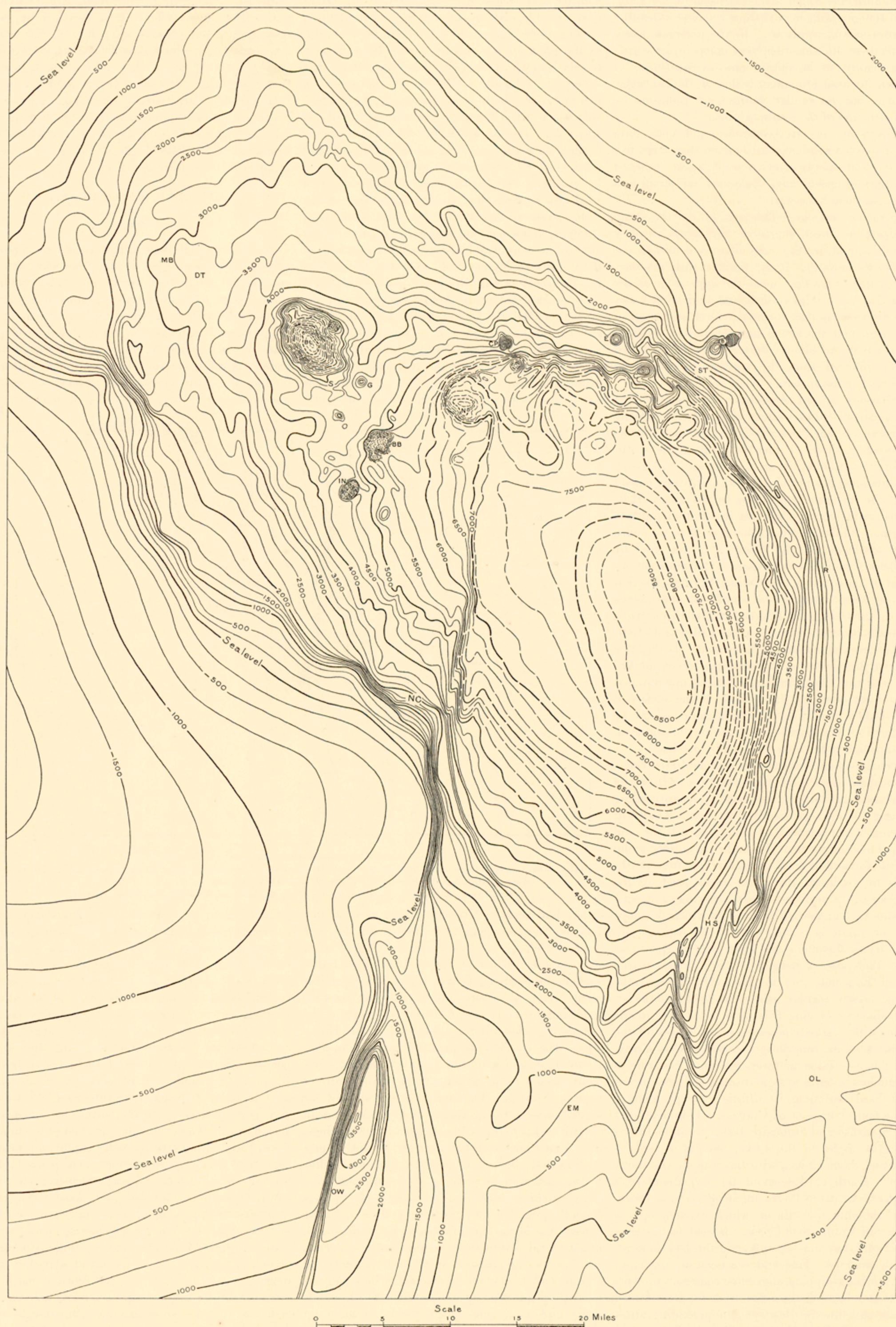
FIG. 1.—Black Hills uplift represented by contours on the surface of Minnekahta limestone. Where the Minnekahta limestone has been removed by erosion the calculated position of the contours is shown by broken lines. Long dashes indicate areas from which Minnekahta and overlying formations have been eroded; short dashes, areas from which all sedimentary rocks have been removed. Contour interval, 250 feet.
