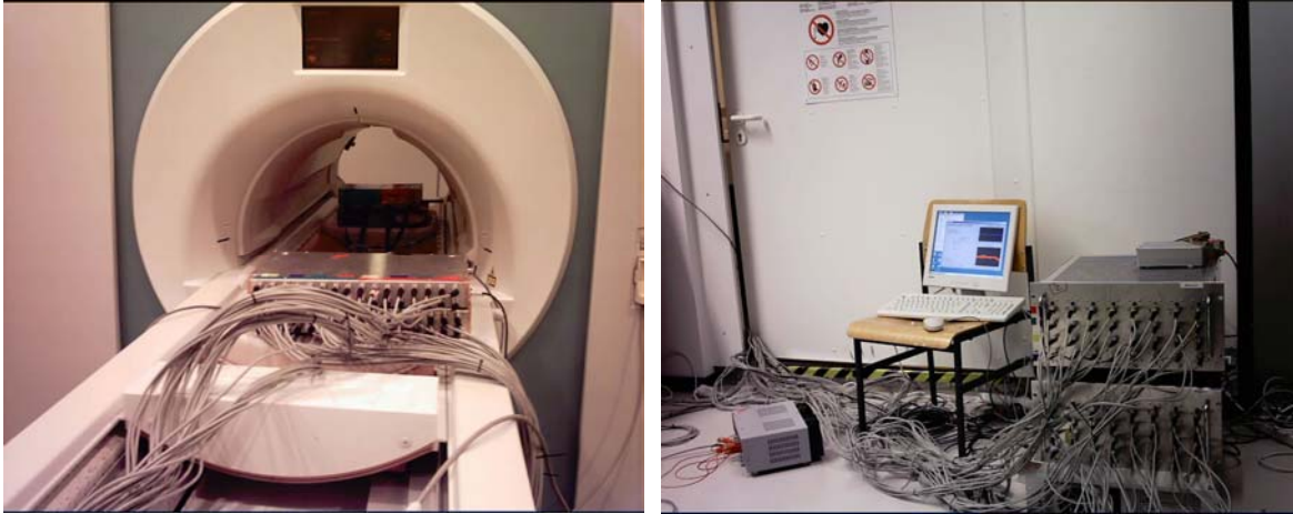
Fig. 4.11 Set up for imaging at 1.5T in Würzburg, Germany. Inside the magnet room (left) showing the coil and phantom on the patient table and the preamplifiers in the foreground; outside the magnet room (right) showing 64 cables run through the scan room door, creating an unshielded environment, connected the 64-channel receiver.
