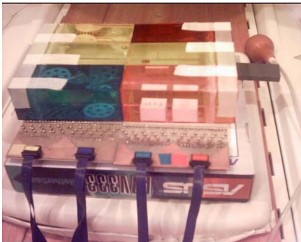
Fig. 4.12 Phantom on 64-channel 1.5T array coil in Würzburg, Germany.
