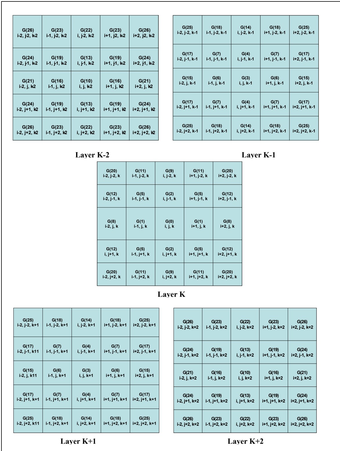
Fig. 2.3–5x5x5 stencil used for the numerical approximation of the square root of the inverse of the covariance
