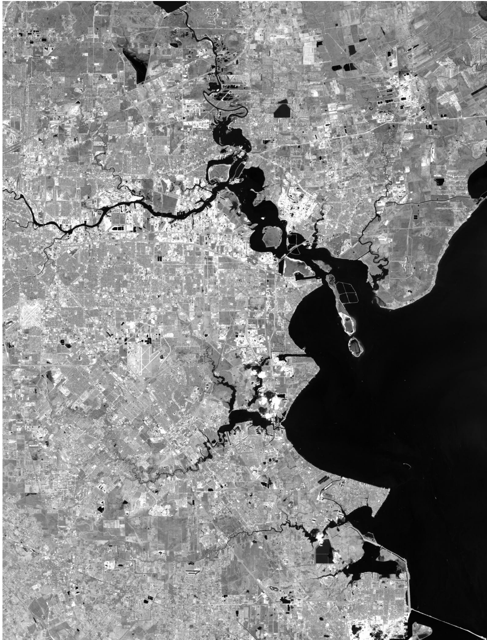
Fig. 22. 1st principal component, result of the PCA, used in the seven band composite image of the vegetation submodel
