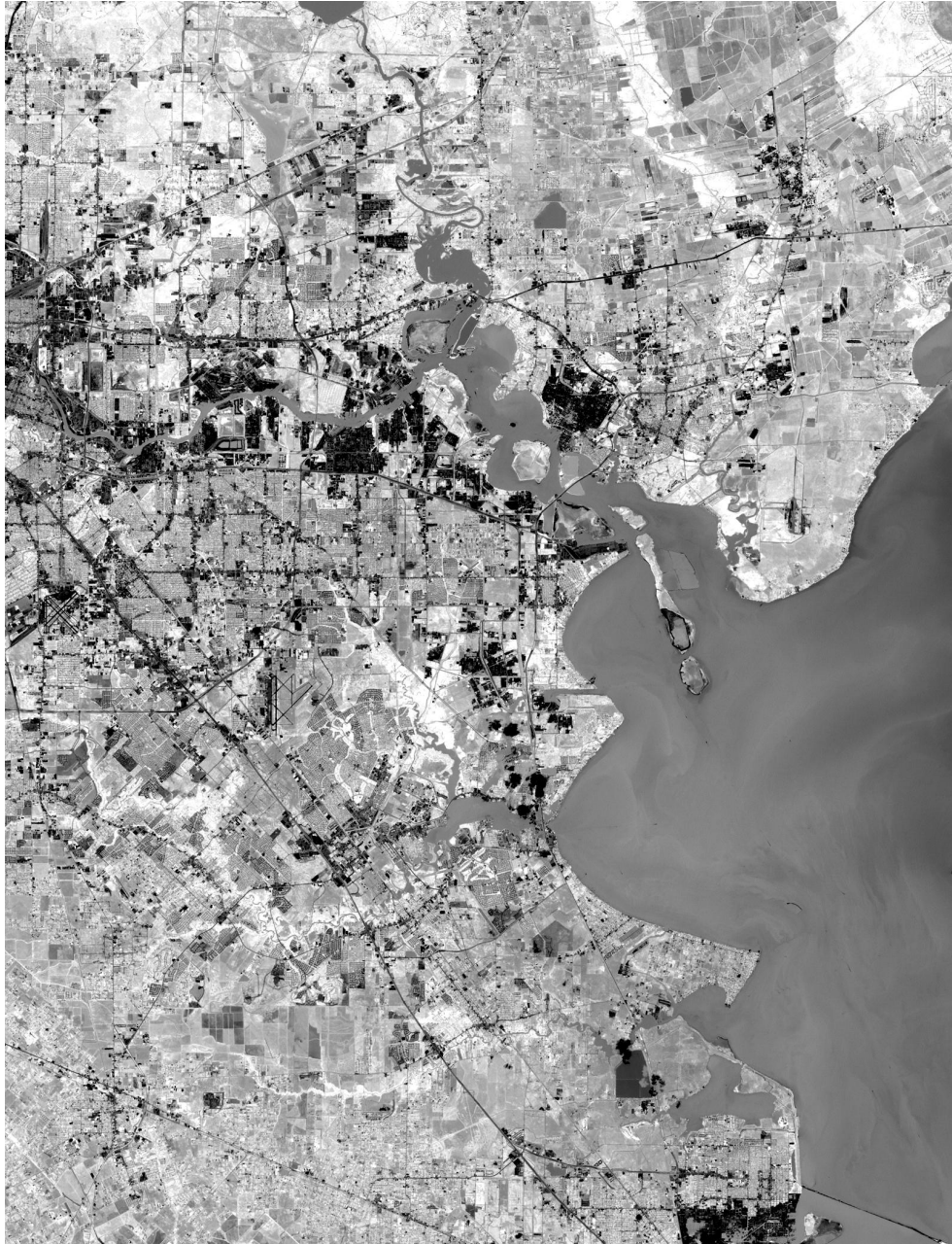
Fig. 23. 2nd principal component, result of the PCA, used in the seven band composite image of the vegetation submodel
