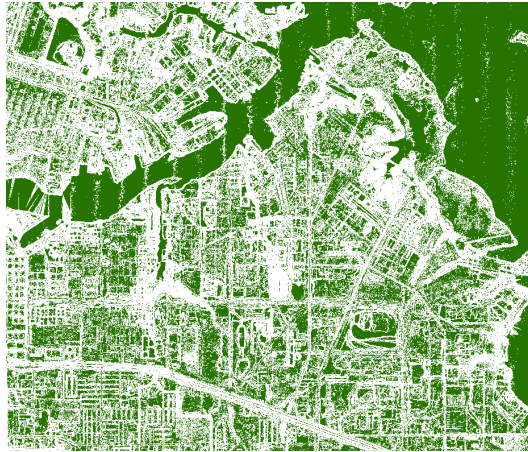
Fig. 9. Slope derived from the DEM with dark areas representing a slope less than one percent
