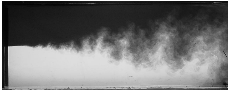
Figure 2.2 Photograph of water channel experiment. The mean flow is from left-to-right and the top fluid is seeded with a Nigrosene dye.
