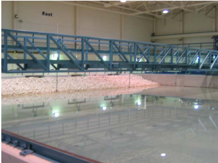
**Figure 4. Parabolic beach and bridge in 3D wave basin**
