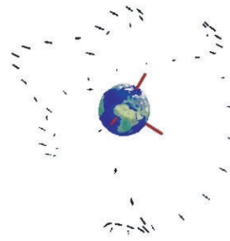
(b) 31-18-57-6-19 FC, i = 63.4^\circ , \omega = 270^\circ , h_p = 22,967.988 \text{ km}
