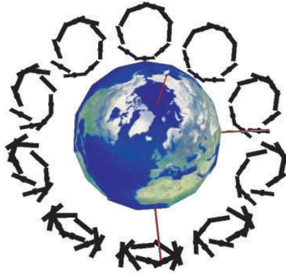
Fig. 24. An 8-1-90-1-90 Flower Constellation with i = 165^\circ , h_p = 3000 \text{ km} , and \omega = 270^\circ . These rings spin about their own axis of symmetry while rigidly rotating about the Flower Constellation axis of symmetry.
