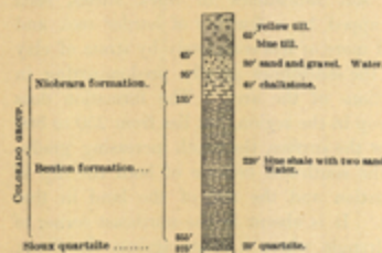
FIG. 3.—Section of well about 7 miles northwest of Milltown, in SW. cor. sec. 14, T. 100 N., R. 60 W.
