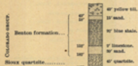
FIG. 5.—Section of well at Wolf Creek.
