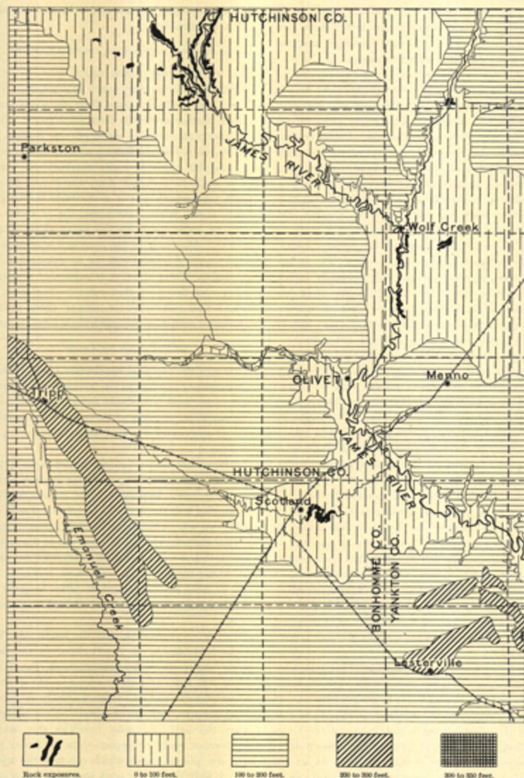
FIG. 6.—Sketch map of Olivet quadrangle showing approximate depths to the bottom of the drift. Water can usually be obtained from sands and gravel at the base of the drift and generally rises many feet in wells.
