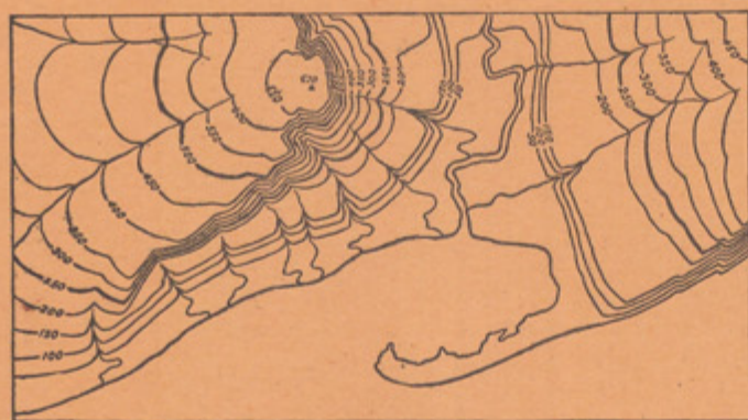
Fig. 1. The upper figure represents a sketch of a river valley, with terraces, and of a high hill encircled by a cliff. These features appear in the map beneath, the slopes and forms of the surface being shown by contours.
