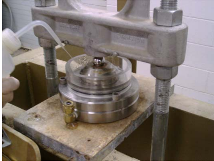
Figure 42: Consolidometer being loaded using the loading frame
