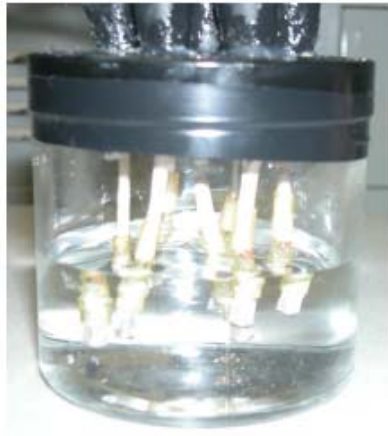
Figure 22: Calibration of thermocouple psychrometer
