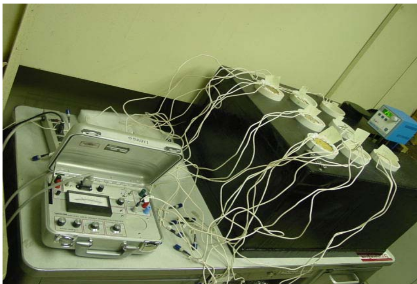
Figure 27: Samples kept in water bath (black box) and measurements being taken by HR-33T (Voltmeter)
