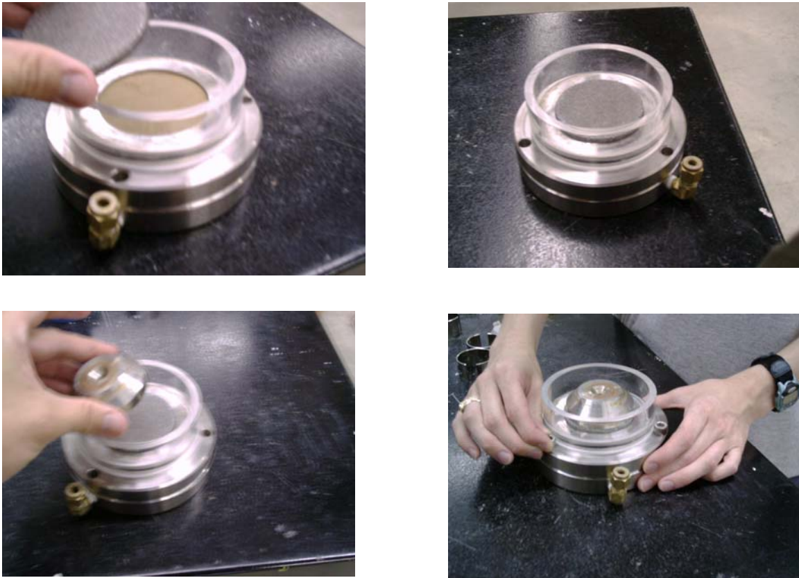
Figure 41: Sample being set inside the consolidometer
