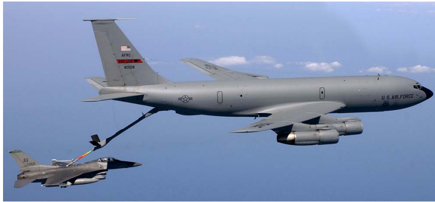
Fig. 1. KC-135 Stratotanker refuels an F-16 Fighting Falcon using the boom method. (U.S. Air Force photo by Tech. Sgt. Mike Buytas)
