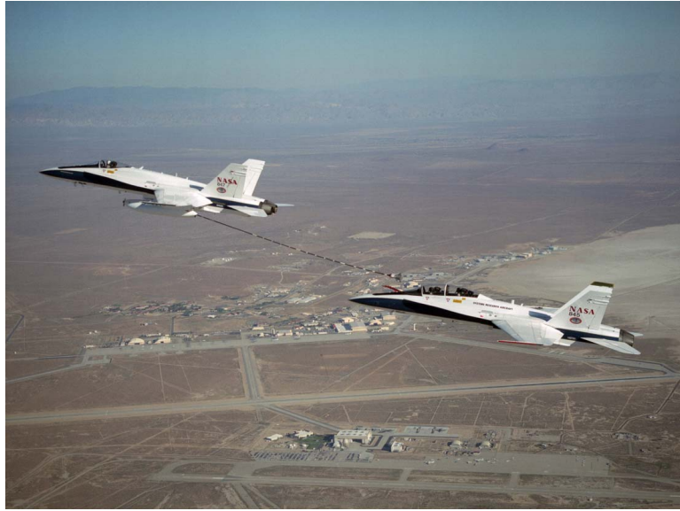
Fig. 5. Two F/A-18 aircraft involved in NASA Dryden’s Automated Aerial Refueling project fly over the California desert. (NASA photo by Carla Thomas)
