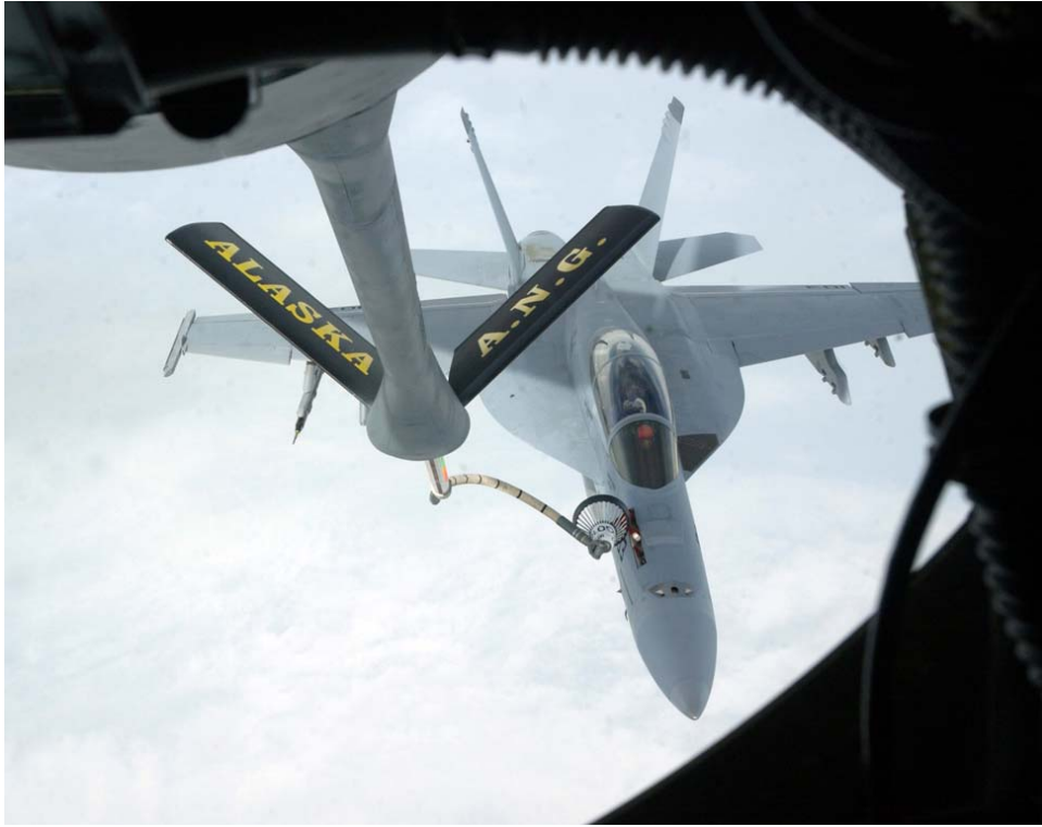
Fig. 4. Navy F/A-18F Super Hornet is refueled by a KC-135R Stratotanker using a boom-drogue adapter. (U.S. Air Force photo by Senior Airman Joshua Strang)
