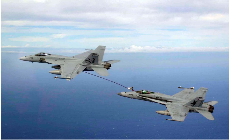
Fig. 3. F/A-18E Super Hornet performs an in flight refueling evolution with an F/A-18C Hornet over the Pacific Ocean using the probe and drogue technique. (U.S. Navy photo by Lt. Perry Solomon)
