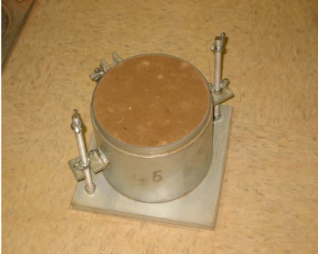
Fig.6.1 Compacted Soil in Mold
