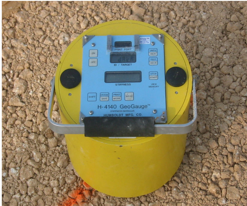
Fig. 2.5 Geogauge in the Field
