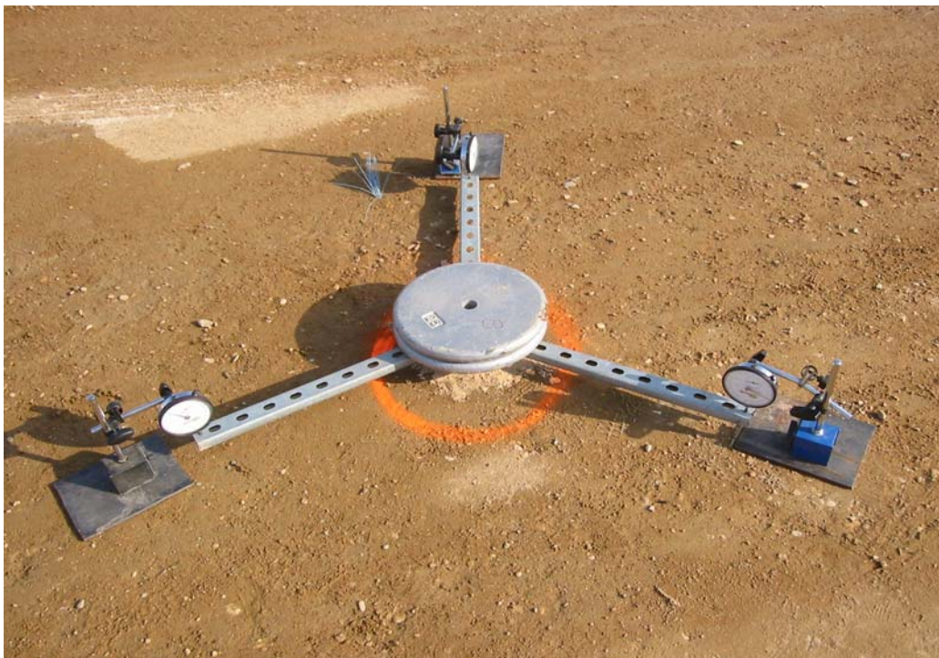
Fig.5.5.b Plate Test in the Field (loading)
