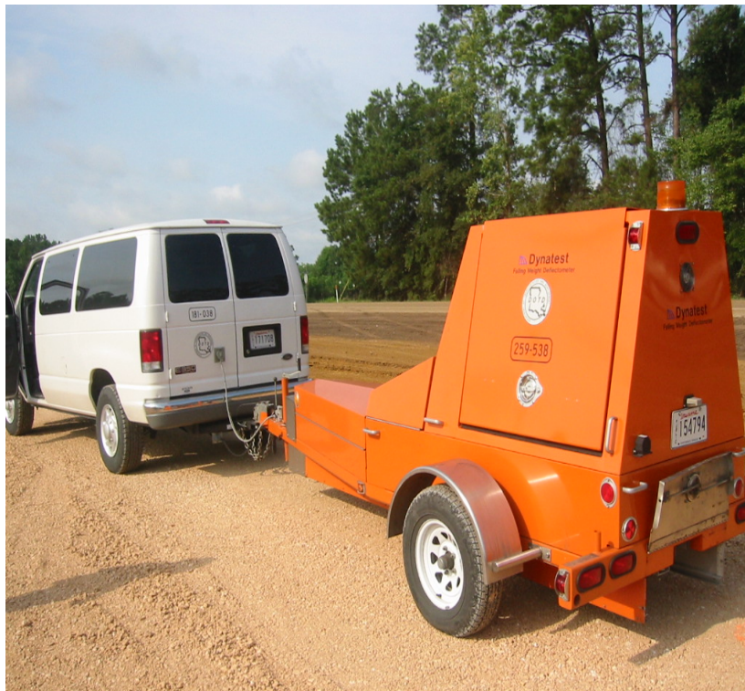
Fig. 2.8 Falling Weight Deflectometer
