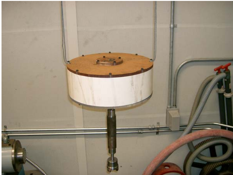
Figure B1 Tumble Mill Assembly Suspended from Cables
