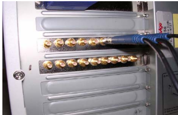
Figure 4.2 Data Acquisition Board Installed in PC
