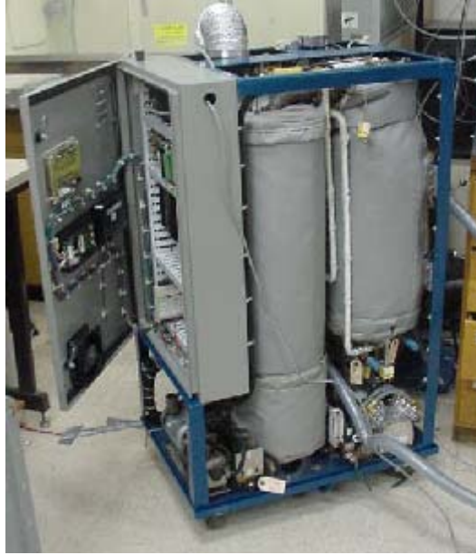
Fig. 4: Adiabatic natural gas reformer that employs POX, SMR, LTS, CO polish, and AGO.
