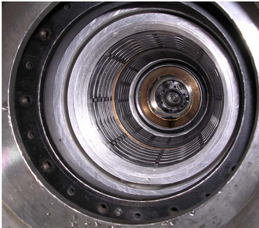
ROTOR REMOVED: 12 BLADED ASSEMBLY
