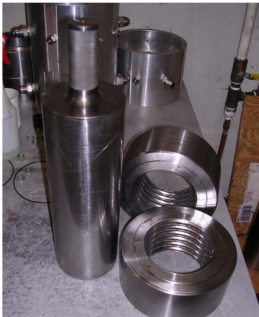
12 BLADED PDS WITH ASSEMBLY MANDREL
