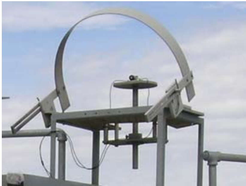
Fig. F-2. Shadow band stand by Eppley with two LI-COR photometric sensors, one placed horizontally and one placed vertically. The position and attachment of this last one was especially customized since the shadow band stand is constructed to receive only one sensor placed horizontally.
