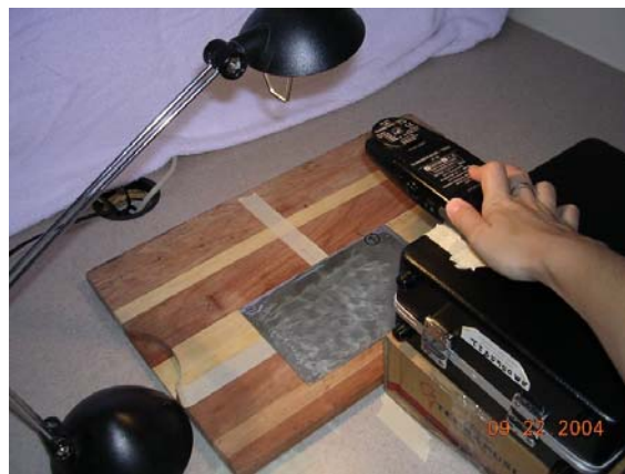
Fig. D-6. Measuring reflected light with light meter facing down half way from the light source.
