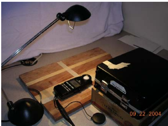
Fig. D-5. Measuring incident light with light meter facing up at wood-board level.
