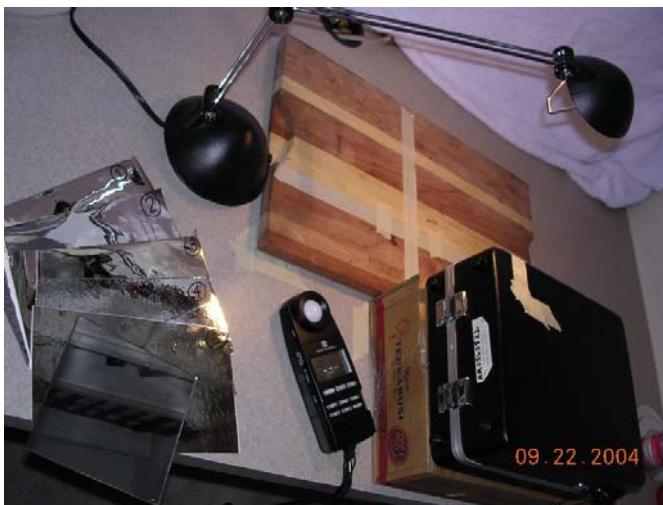
Fig. D-2. Setup for experiment to measure reflectivity of different types of “Silver III” mountings.
