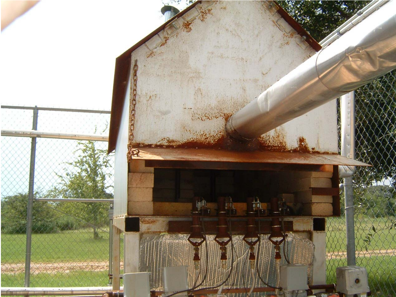
Figure A.29 The steam produced from the boiler was superheated using the super-heater before entering the jet ejector as motive stream.
