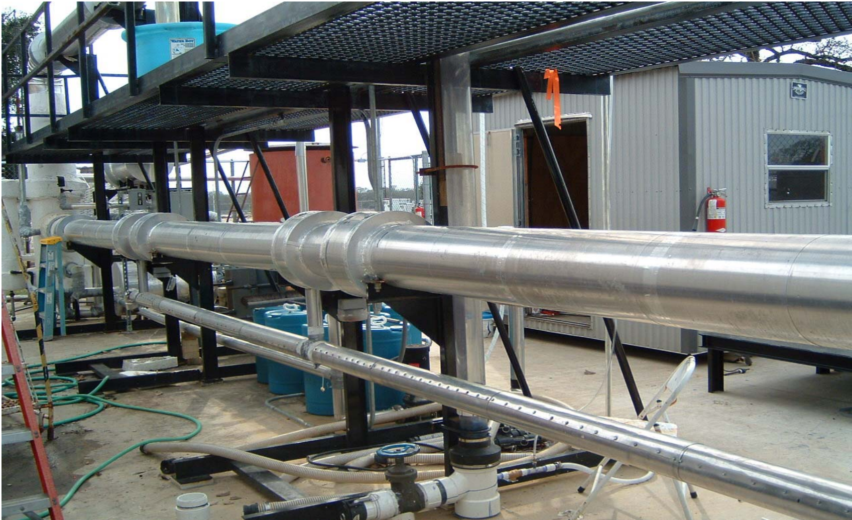
Figure A.30 A closer look of the desalination unit, showing the three jet ejectors connected in series.
