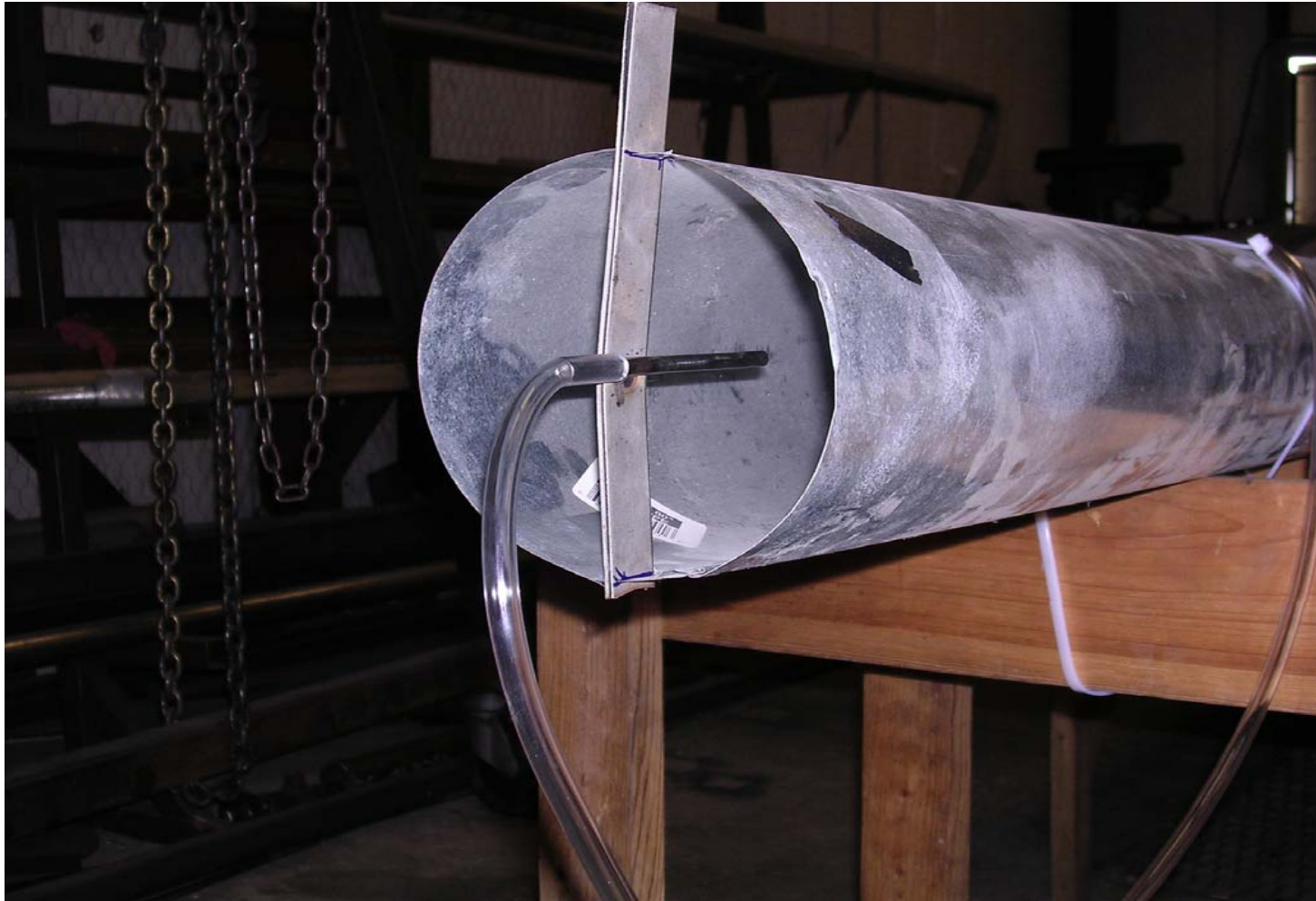
Figure A.25 The experimental setup showing the pitot-tube placed at the outlet of the jet ejector to measure the dynamic pressure.
