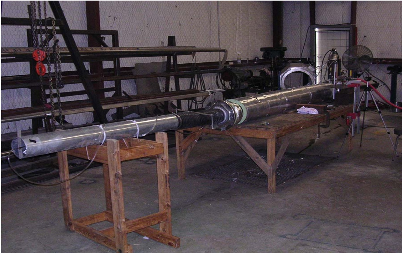
Figure A.22 The experimental setup showing jet ejector and the extension at the outlet along with the pinch valve.
