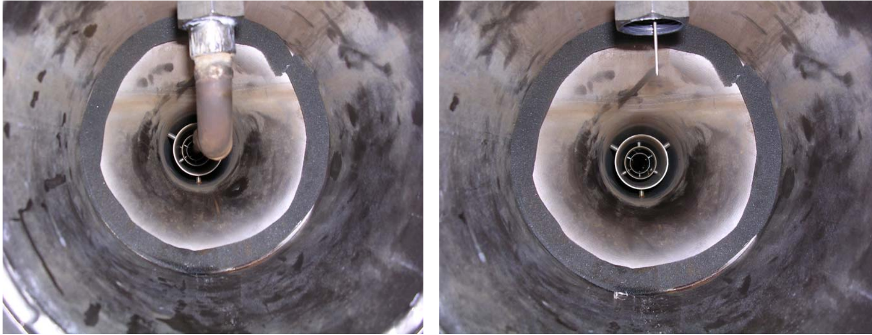
Figure A.27 The inside view of the jet ejector showing the mixing vanes and the nozzle. (a) The left picture shows the nozzle pointing towards the diffuser is placed at the center of the mixing vanes. (b) The right picture shows the three internal mixing vanes located in the diffuser section of the jet ejector for proper mixing of motive and propelled streams.
