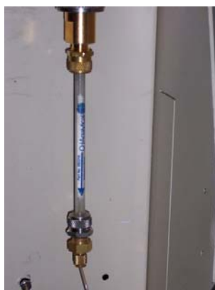
Fig. 5. Air tube placement in the P&T unit
