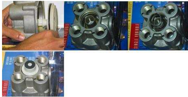
Fig. 5. Relay valve parts getting assembled
