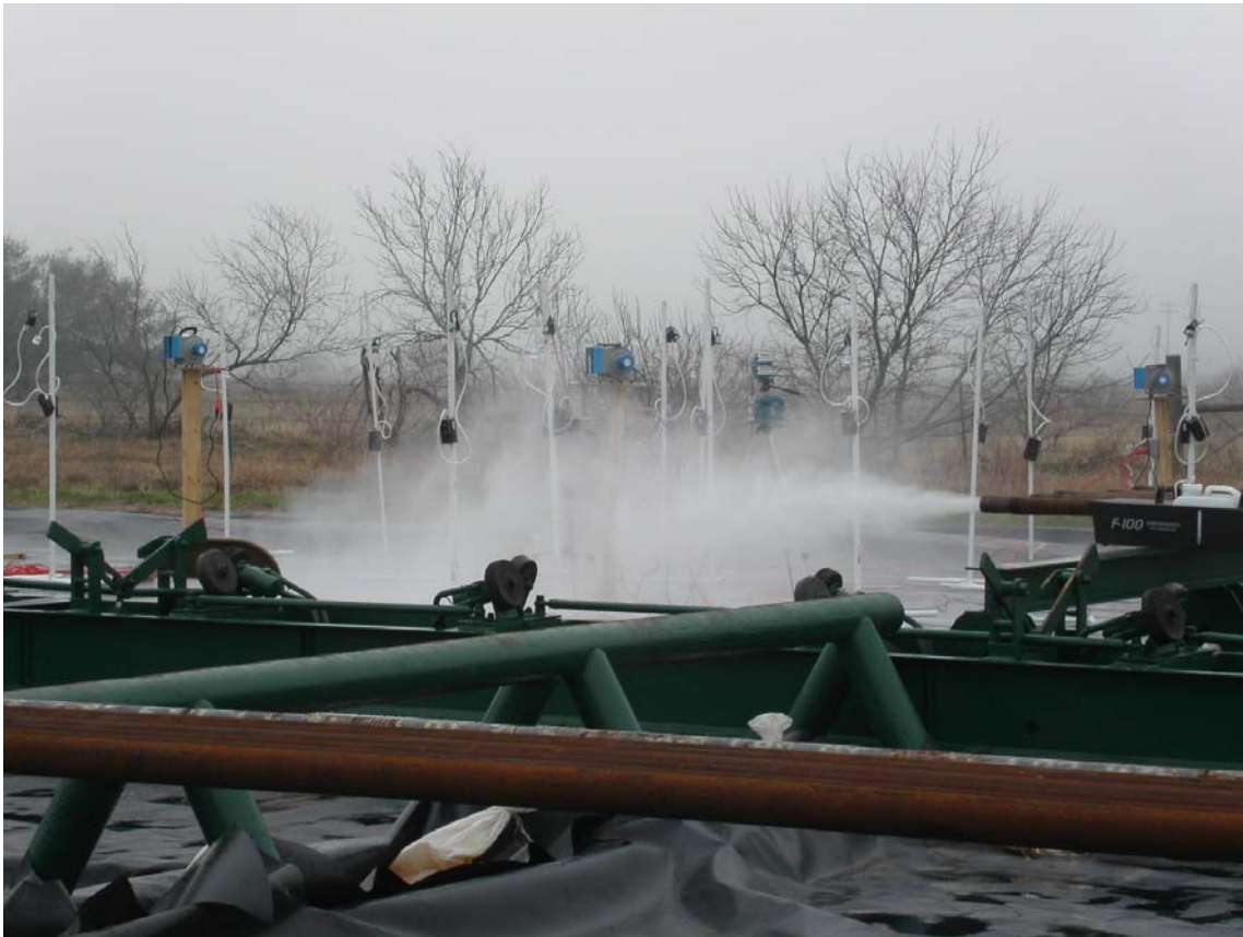
Figure 3. Scale released during dry pipe cleaning experiment.
