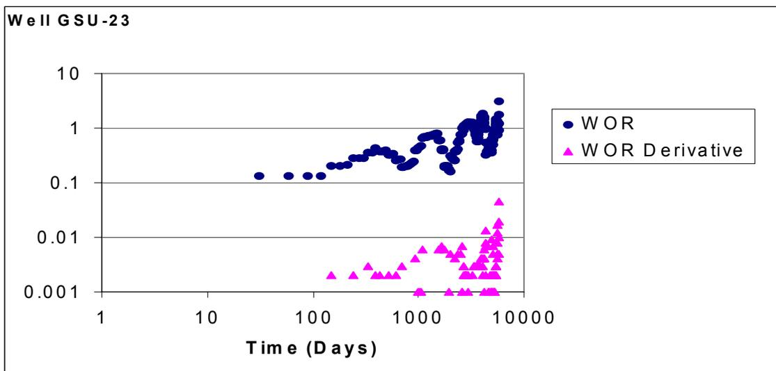
**Fig. 67 -WOR and WOR Derivative for Well GSU-23: Experiencing Normal Displacement with High WOR.**
