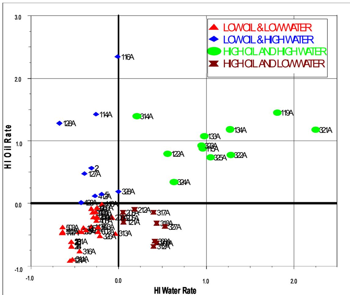
**Fig. 11 - Cross-Plot Showing the Production Heterogeneity Index for Oil and Water in 64 Active Wells of Germania Spraberry Unit.**
