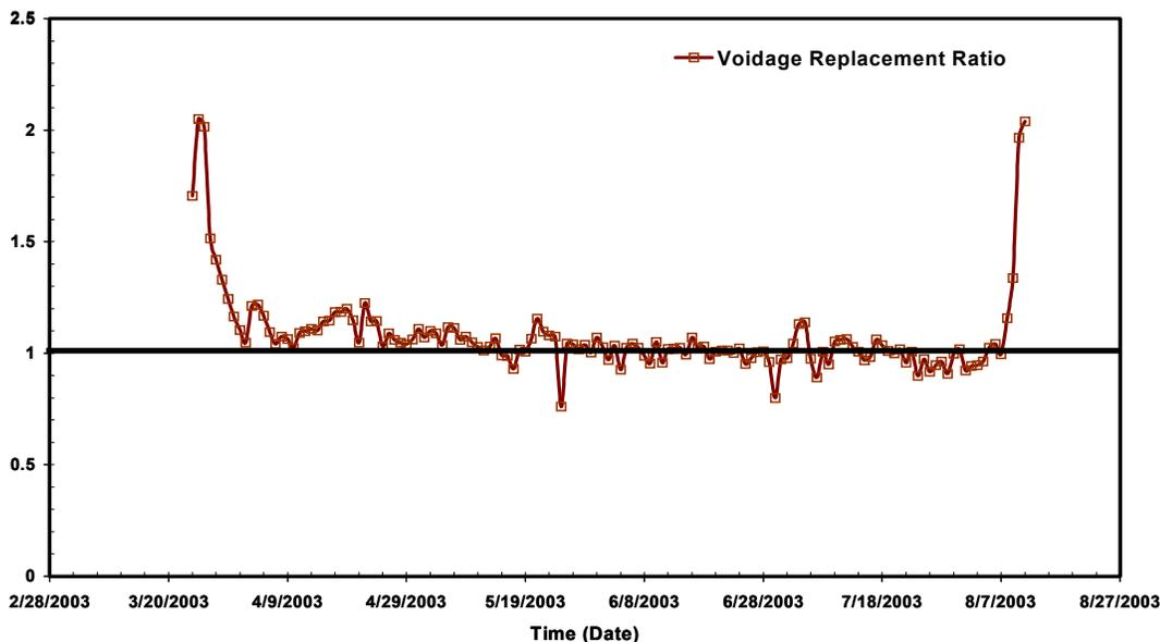
**Fig. 15 -Voidage Replacement Ratio for the Second Period of Injection**
