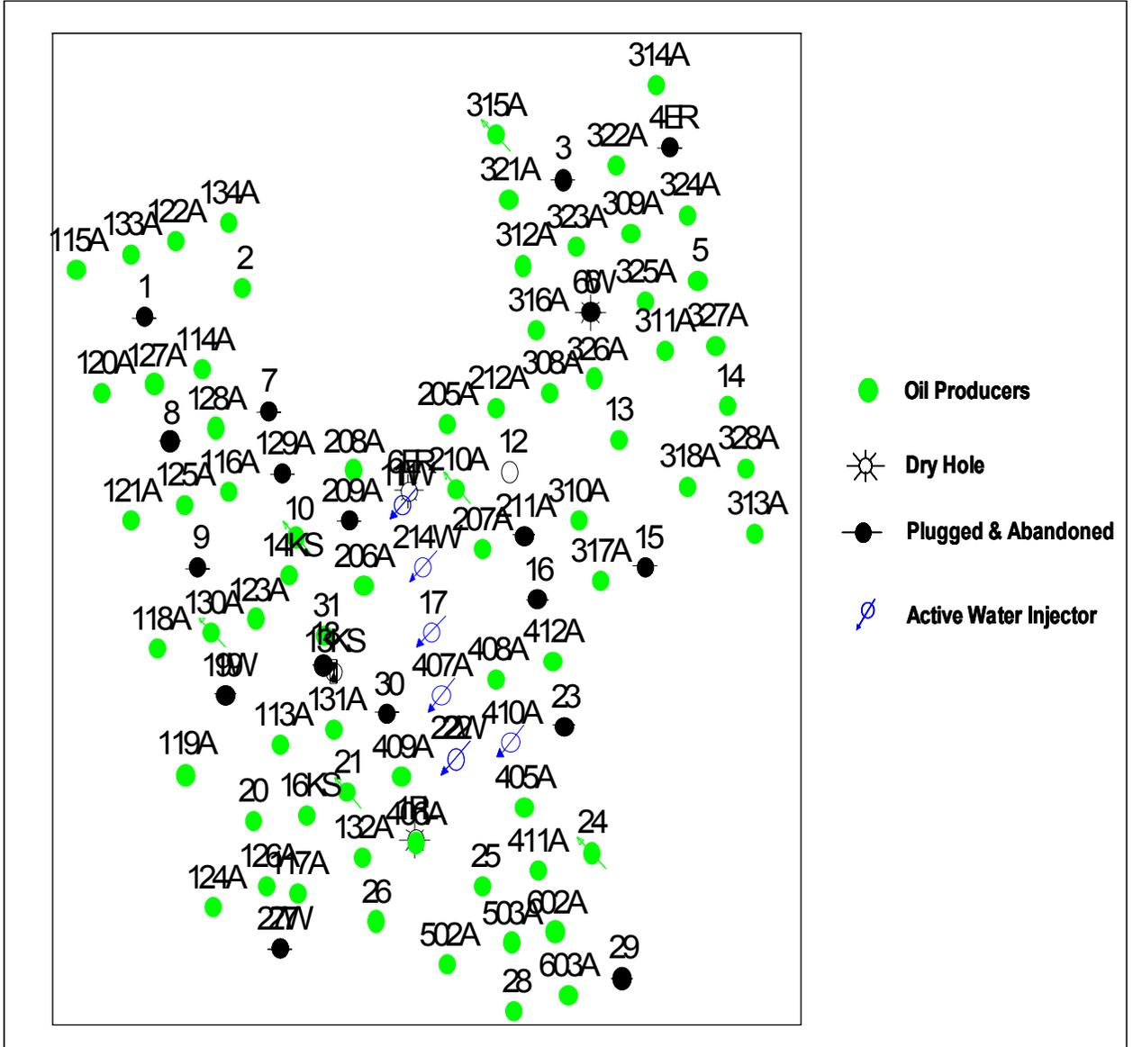
Fig. 2 – Location of New Water Injectors Wells in Germania Spraberry Unit.
