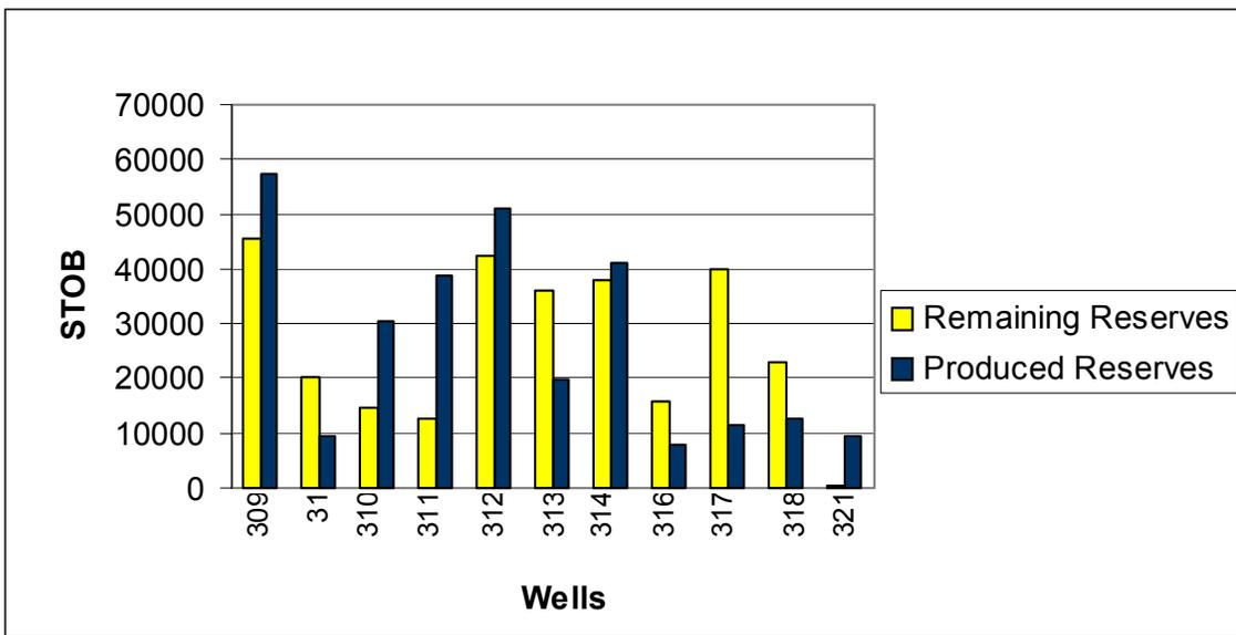
**Fig. 87 - Remaining and Produced Reserves for Wells GSU-309,GSU-31,GSU-310,GSU-311,GSU-312,GSU-313,GSU-314,GSU-316,GSU-317,GSU-318, and GSU-321.**
