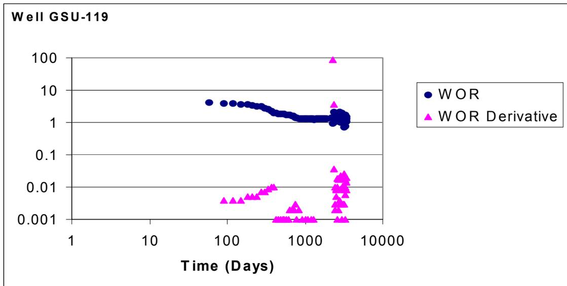
**Fig. 53 -WOR and WOR Derivative for Well GSU-119: Experiencing Near Wellbore Water Channeling.**
