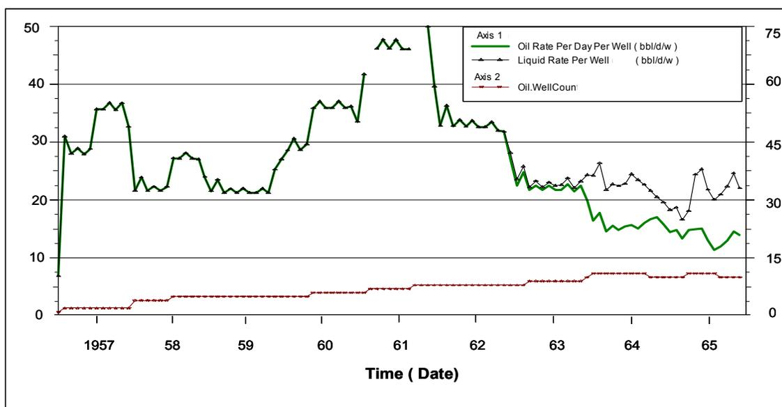
**Fig. 5 -Oil Rate per well, Liquid Rate per Well and Active Wells During Primary Depletion for Germania Spraberry Unit.**
