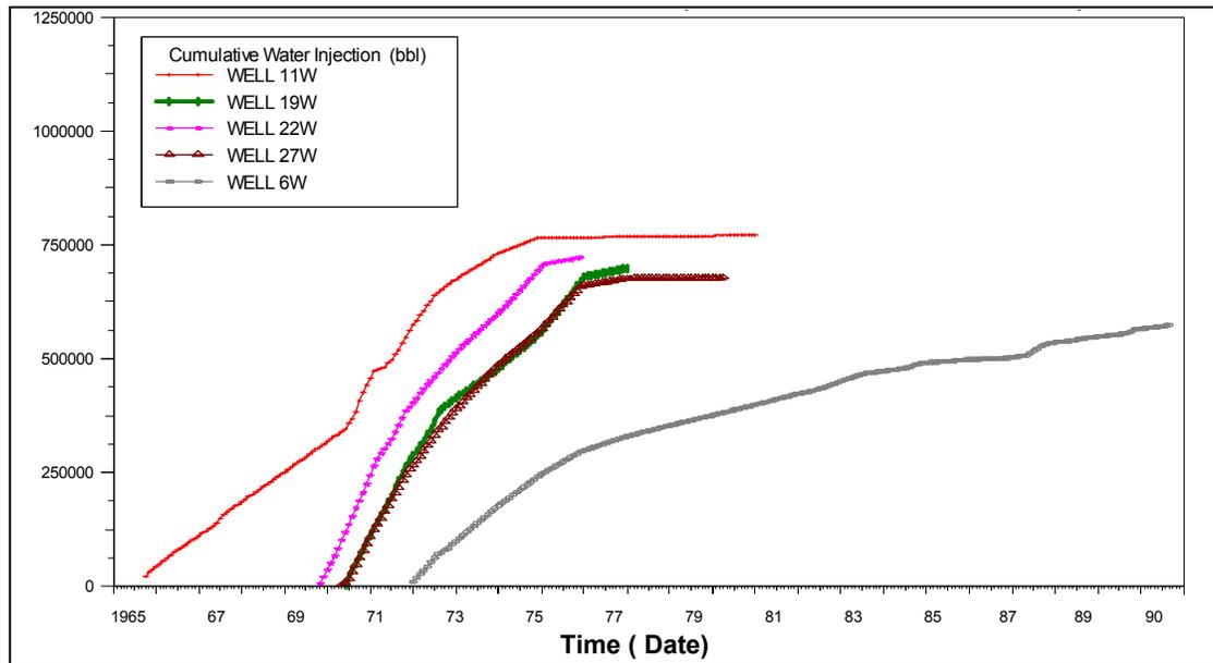
**Fig. 7 - Cumulative Water Injection for the Five Wells Injecting from 1965 to 1990.**
