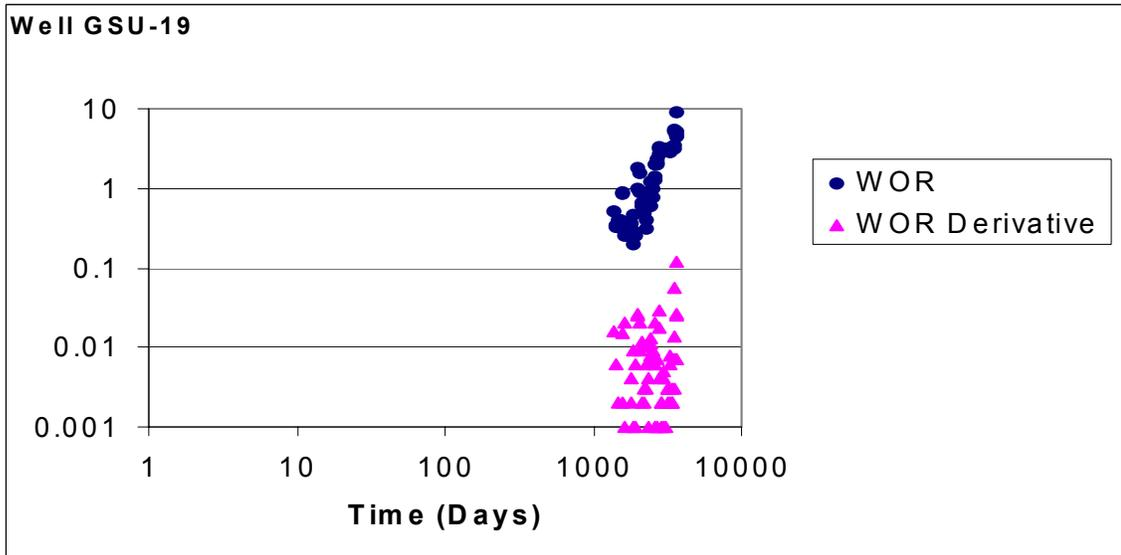
**Fig. 60 -WOR and WOR Derivative for Well GSU-19: Experiencing Rapid Channeling.**
