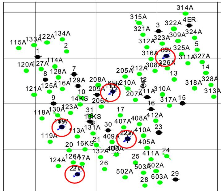
**Fig. 6 -Base Map of Germania Spraberry Unit Showing the Wells Injecting Water from 1965 to 1990.**
