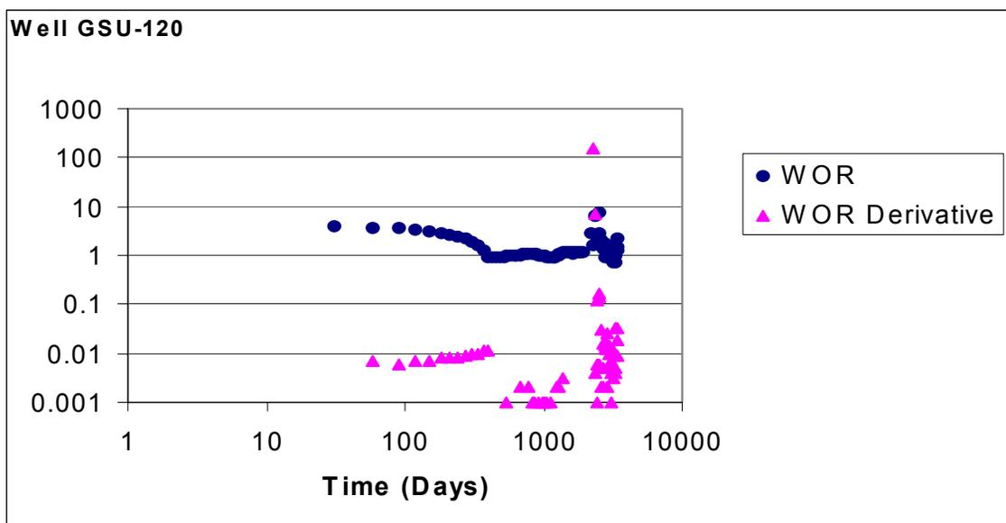
**Fig. 54 -WOR and WOR Derivative for Well GSU-120: Experiencing Near Wellbore Water Channeling**
