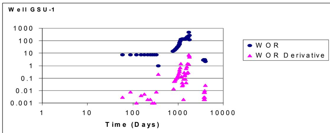
**Fig. 48 -WOR and WOR Derivative for Well GSU-1: Experiencing Near Wellbore Water Channeling.**
