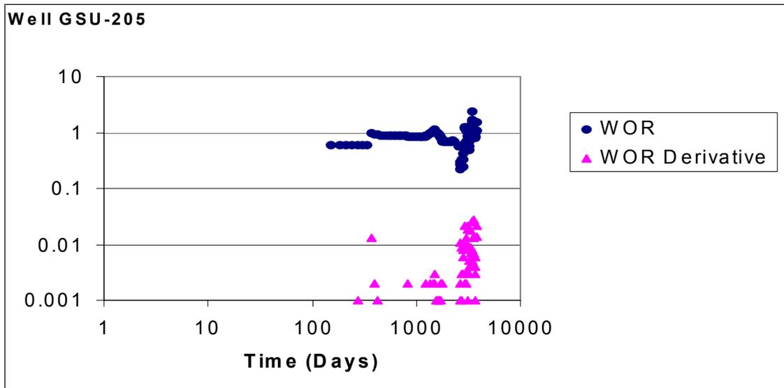
**Fig. 71 -WOR and WOR Derivative for Well GSU-205: Experiencing Normal Displacement with High WOR.**
