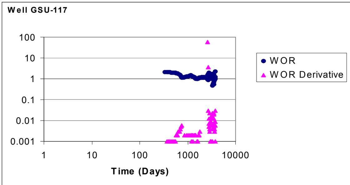
**Fig. 51 -WOR and WOR Derivative for Well GSU-117: Experiencing Near Wellbore Water Channeling.**
