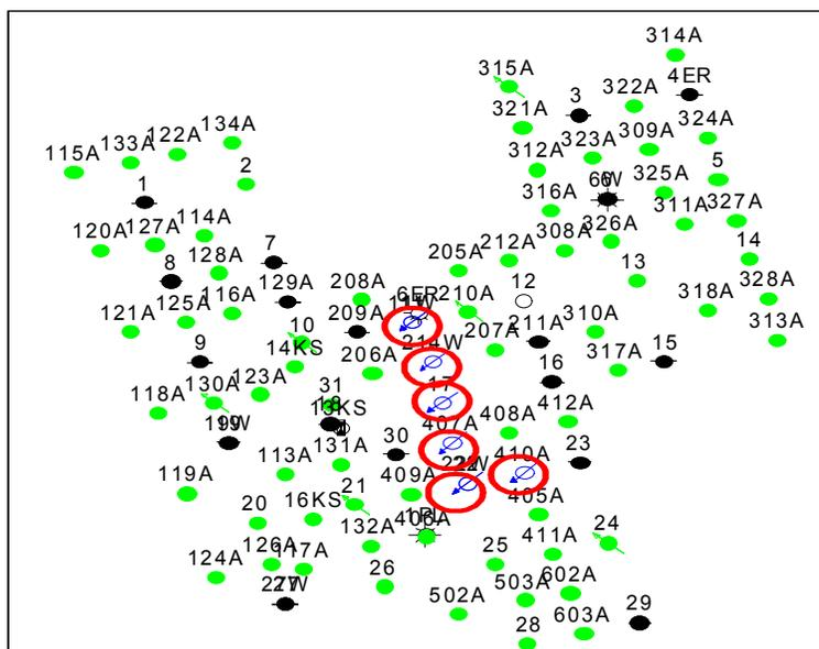
**Fig. 9 -Base Map of Germania Spraberry Unit Showing Wells Injecting Water Under the New Injection Pattern (January 2003).**
