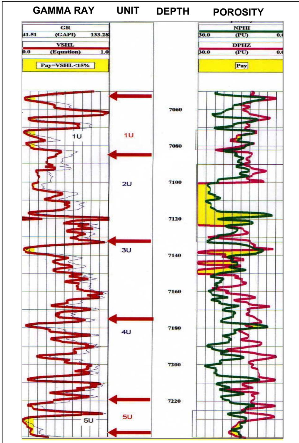
Fig. 3 – Type log for Upper Spraberry Interval. Well GSU-1.
