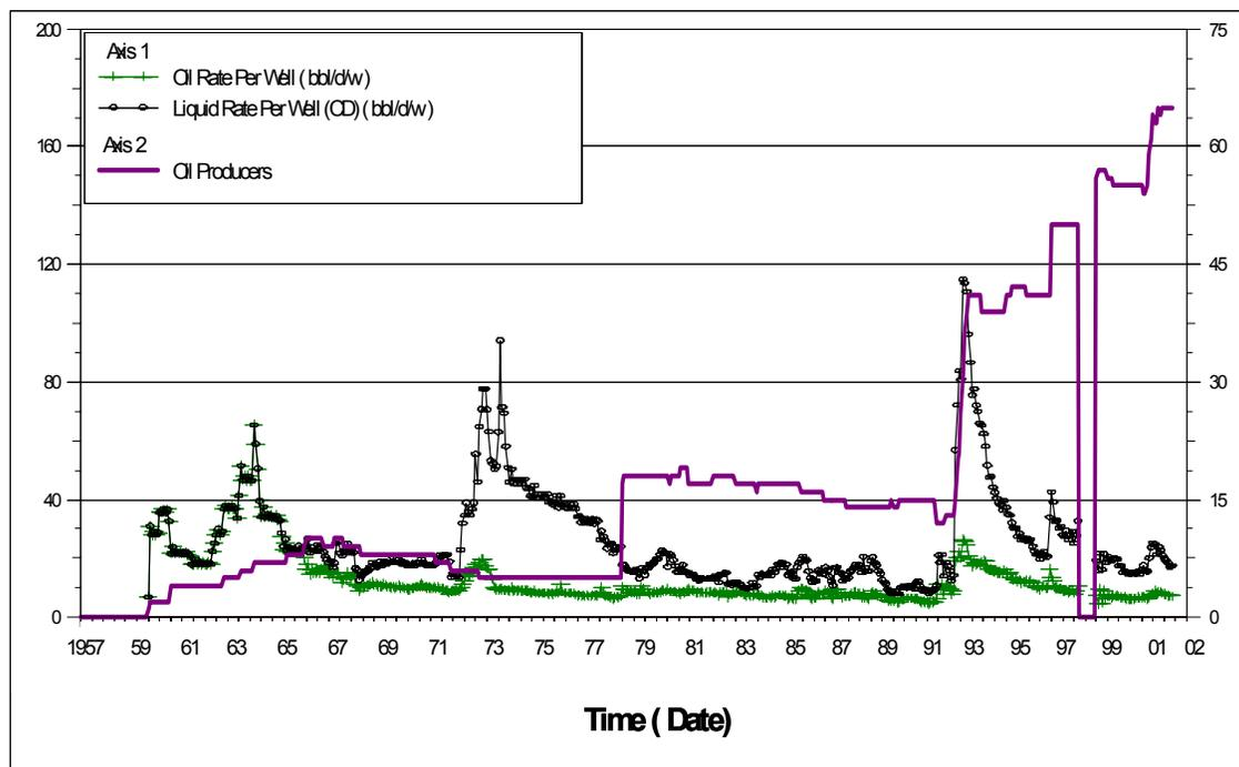
**Fig. 10 -Oil Rate per well, Liquid Rate per Well and Active Wells During Primary and Secondary Depletion for Germania Spraberry Unit.**
