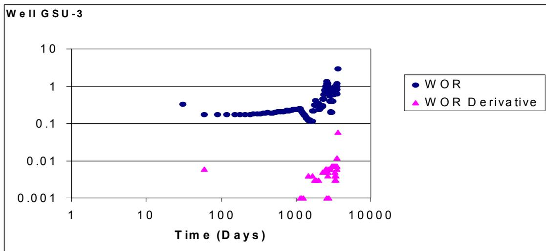
**Fig. 57 -WOR and WOR Derivative for Well GSU-3: Experiencing Water Coning with Late Time Channeling.**
