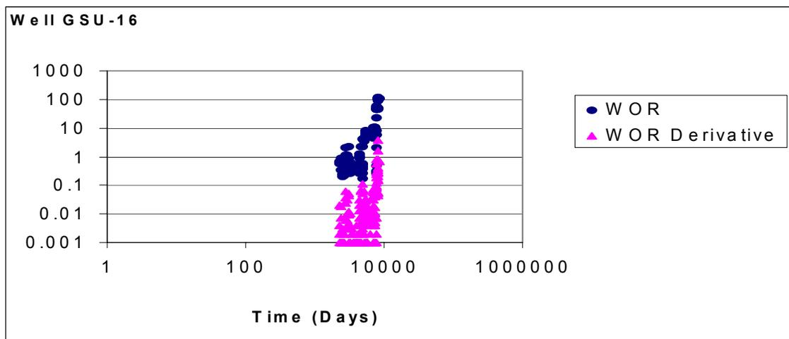
**Fig. 59 -WOR and WOR Derivative for Well GSU-16: Experiencing Rapid Channeling.**
