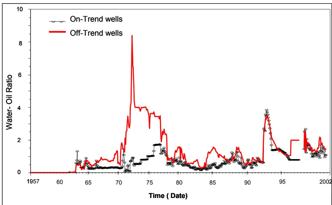
**Fig. 18 -Average Water-Oil ratio for On-trend and Off-trend wells.**
