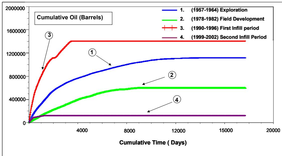
**Fig. 31 -Cumulative Oil Production for Different Drilling Programs During the Development of Germania Spraberry Unit.**
