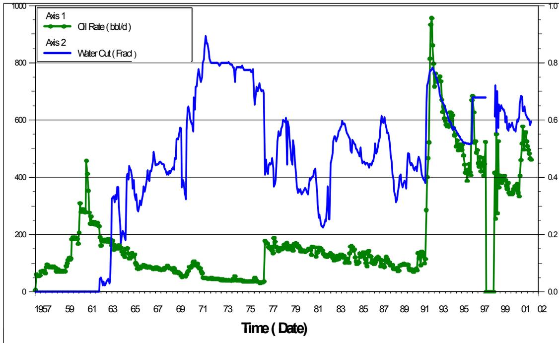
**Fig. 8 -Oil Rate and Water Cut during Primary and Secondary Depletion of Germania Spraberry Unit.**
