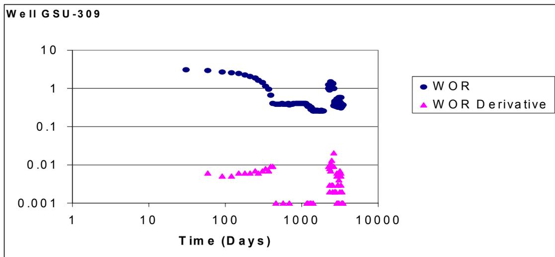
**Fig. 56 -WOR and WOR Derivative for Well GSU-309: Experiencing Water Coning with Late Time Channeling.**
