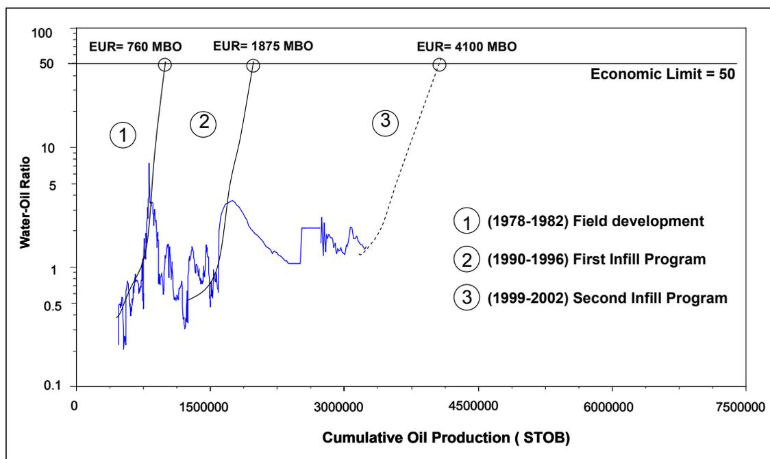
**Fig. 92 - WOR behavior and Cumulative Oil Production Due to Infill Drilling and Waterflooding in Germania Spraberry Unit.**
