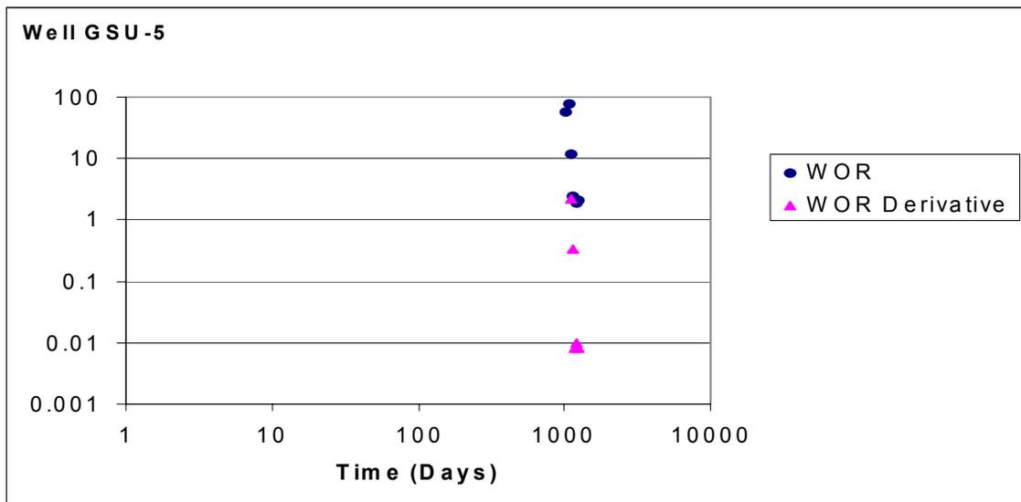
**Fig. 64 -WOR and WOR Derivative for Well GSU-5: Experiencing Rapid Channeling.**
