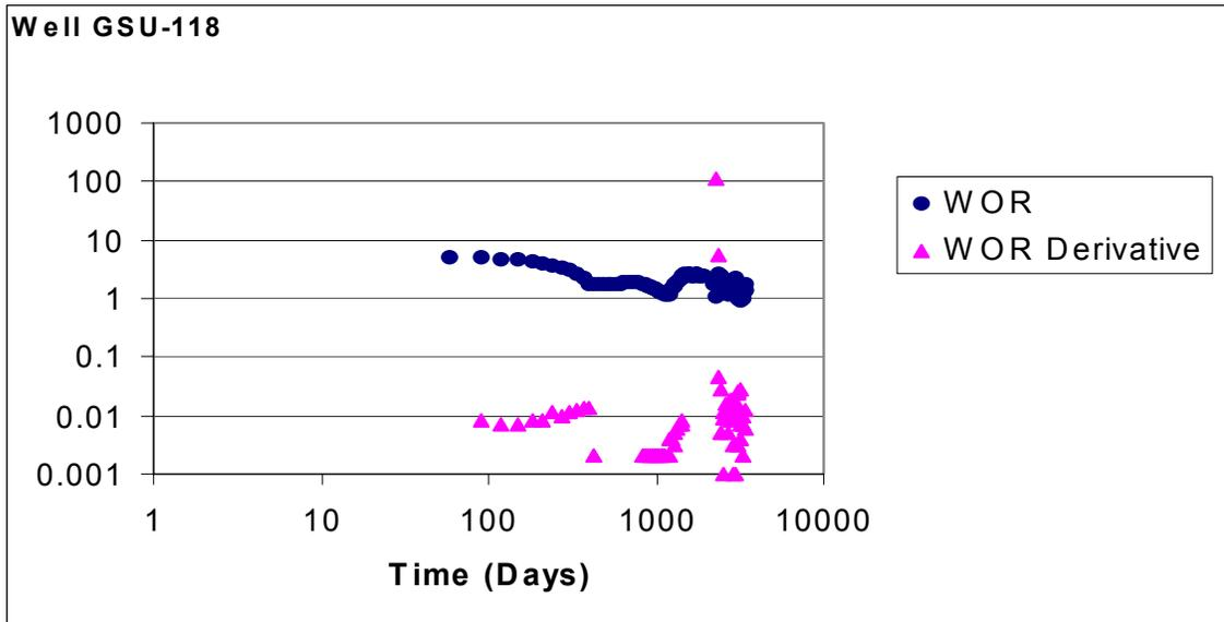
**Fig. 52 -WOR and WOR Derivative for Well GSU-118: Experiencing Near Wellbore Water Channeling.**
