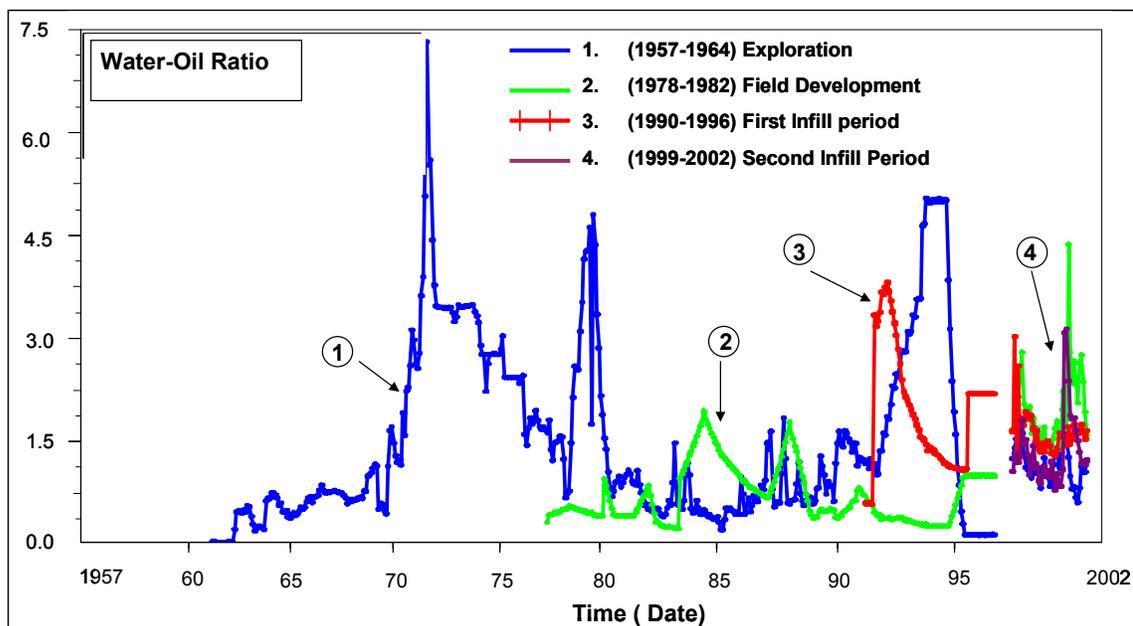
**Fig. 30 -Historical Water-Oil Ratio for Different Drilling Programs During the Development of Germania Spraberry Unit.**
