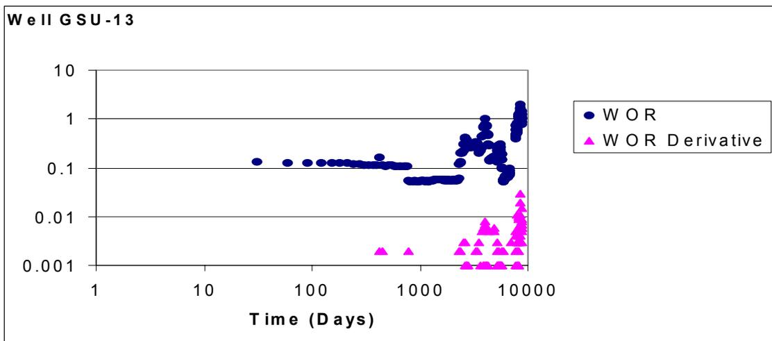
**Fig. 66 -WOR and WOR Derivative for Well GSU-13: Experiencing Normal Displacement with High WOR.**
