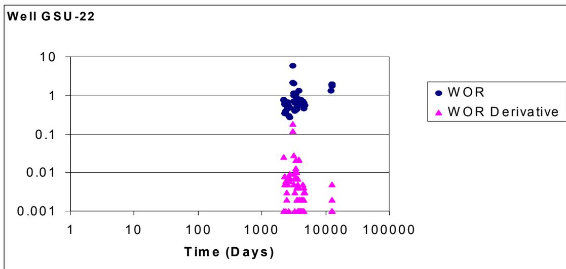
**Fig. 62 -WOR and WOR Derivative for Well GSU-22: Experiencing Rapid Channeling**
