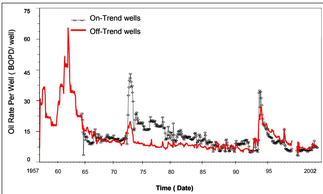
**Fig. 17 -Oil Rate per Well for On-trend and Off-trend Wells.**
