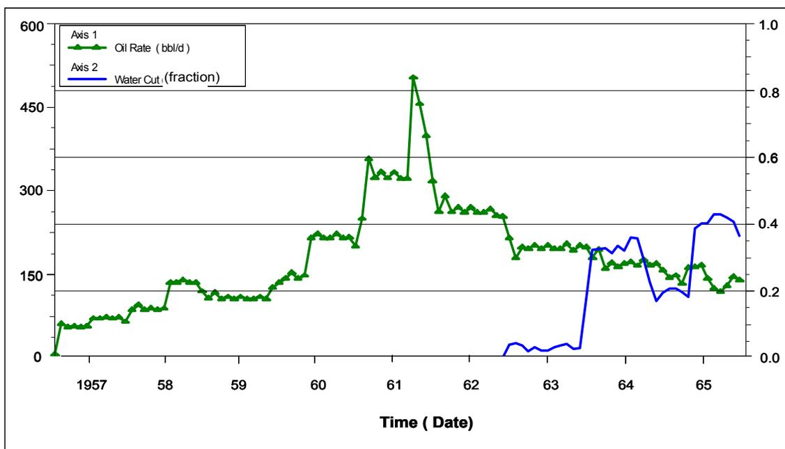
**Fig. 4 -Oil Rate and Water Cut During Primary Depletion of Germania Spraberry Unit.**
