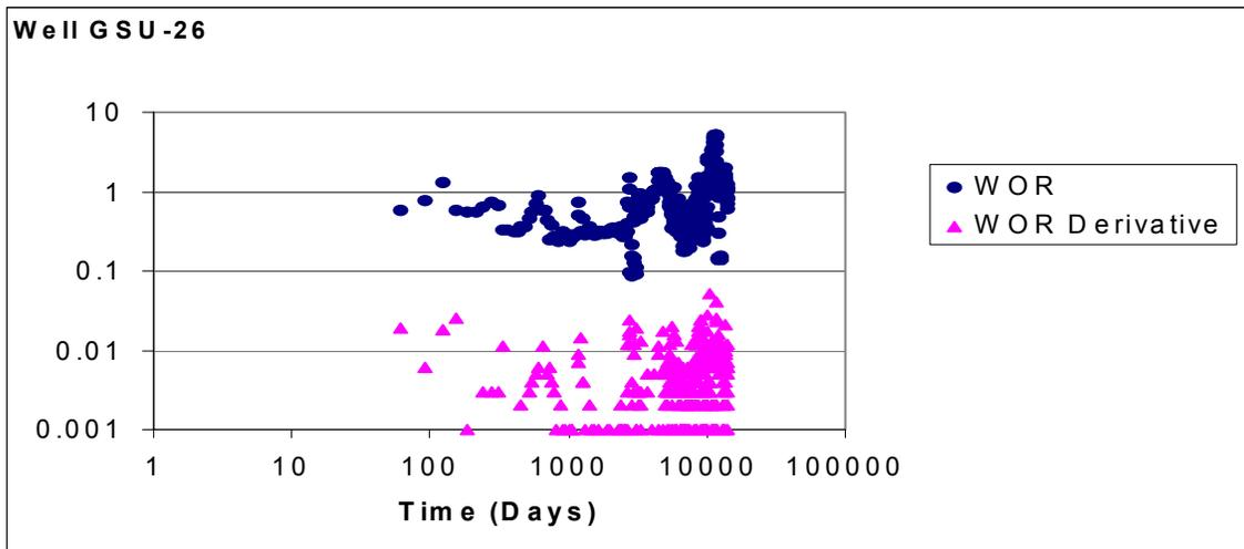
**Fig. 69 -WOR and WOR Derivative for Well GSU-26: Experiencing Normal Displacement with High WOR.**
