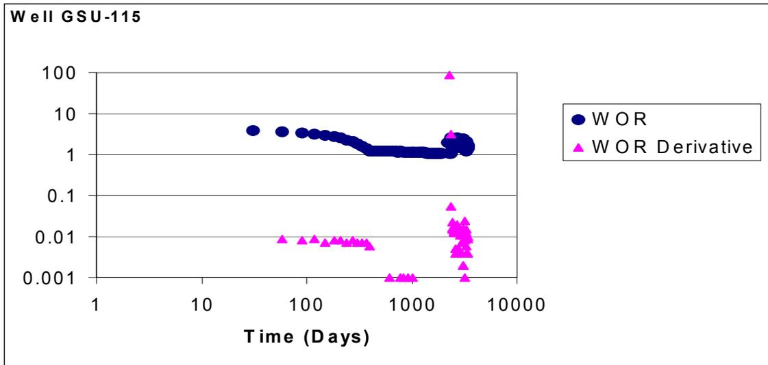
**Fig. 50 -WOR and WOR Derivative for Well GSU-115: Experiencing Near Wellbore Water Channeling.**
