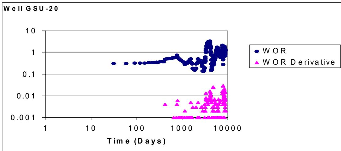
**Fig. 65 -WOR and WOR Derivative for Well GSU-20: Experiencing Normal Displacement with High WOR.**
