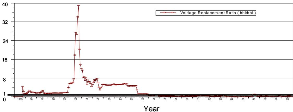
**Fig. 14 -Voidage Replacement Ratio for the First Period of Injection**
