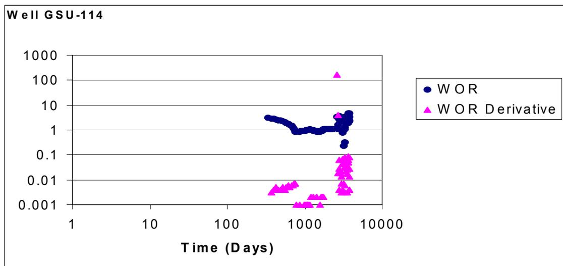
**Fig. 49 -WOR and WOR Derivative for Well GSU-114: Experiencing Near Wellbore Water Channeling.**
