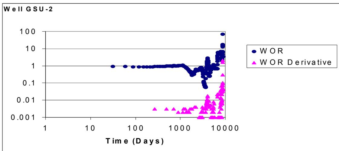
**Fig. 55 -WOR and WOR Derivative for Well GSU-2: Experiencing Near Wellbore Water Channeling.**
