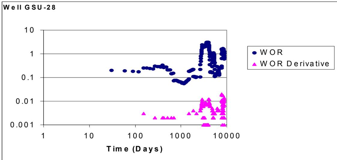
**Fig. 70 -WOR and WOR Derivative for Well GSU-28: Experiencing Normal Displacement with High WOR.**
