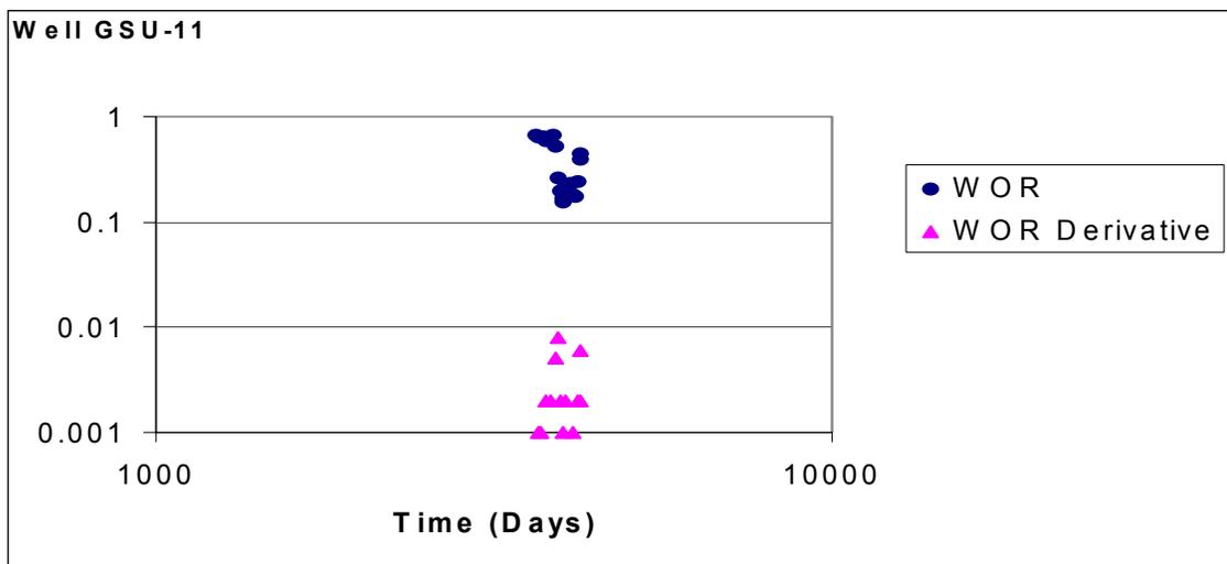
**Fig. 58 -WOR and WOR Derivative for Well GSU-11: Experiencing Rapid Channeling.**
