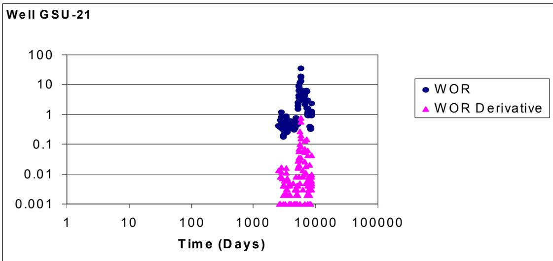
**Fig. 61 -WOR and WOR Derivative for Well GSU-21: Experiencing Rapid Channeling.**
