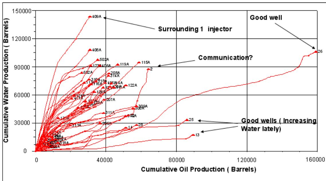
**Fig. 73 -Scatter Plot Showing the Performance of Cumulative Oil vs. Cumulative Water for Active Wells in Germania Spraberry Unit.**
