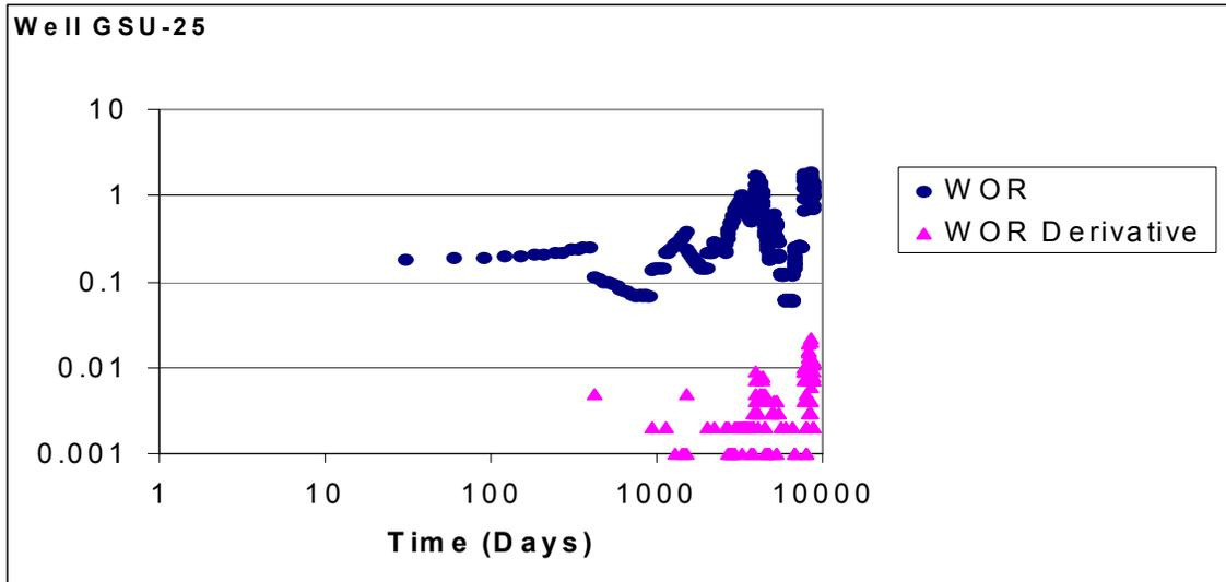
**Fig. 68 -WOR and WOR Derivative for Well GSU-25: Experiencing Normal Displacement with High WOR.**
