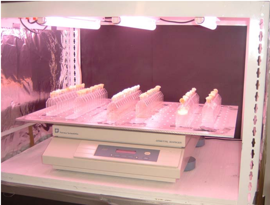
FIGURE 11. Cyanobacteria growth chamber. Another orbital shaker is located below.
