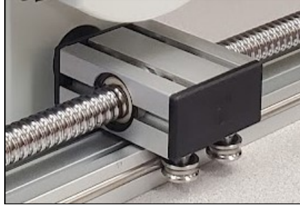
Figure 22. Roller Bearings on Stage in Contact with Precision Rod.
