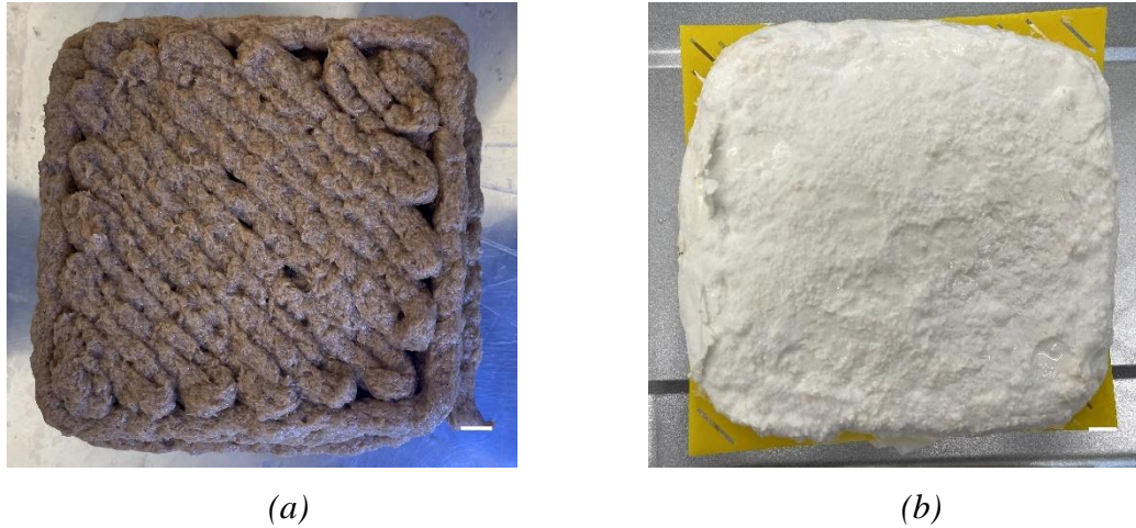
Figure 35: Images of samples: (a) After 3D printing, scale bar is 1 cm; (b) 3D printed after undergoing secondary colonization, scale bar is 1 cm
