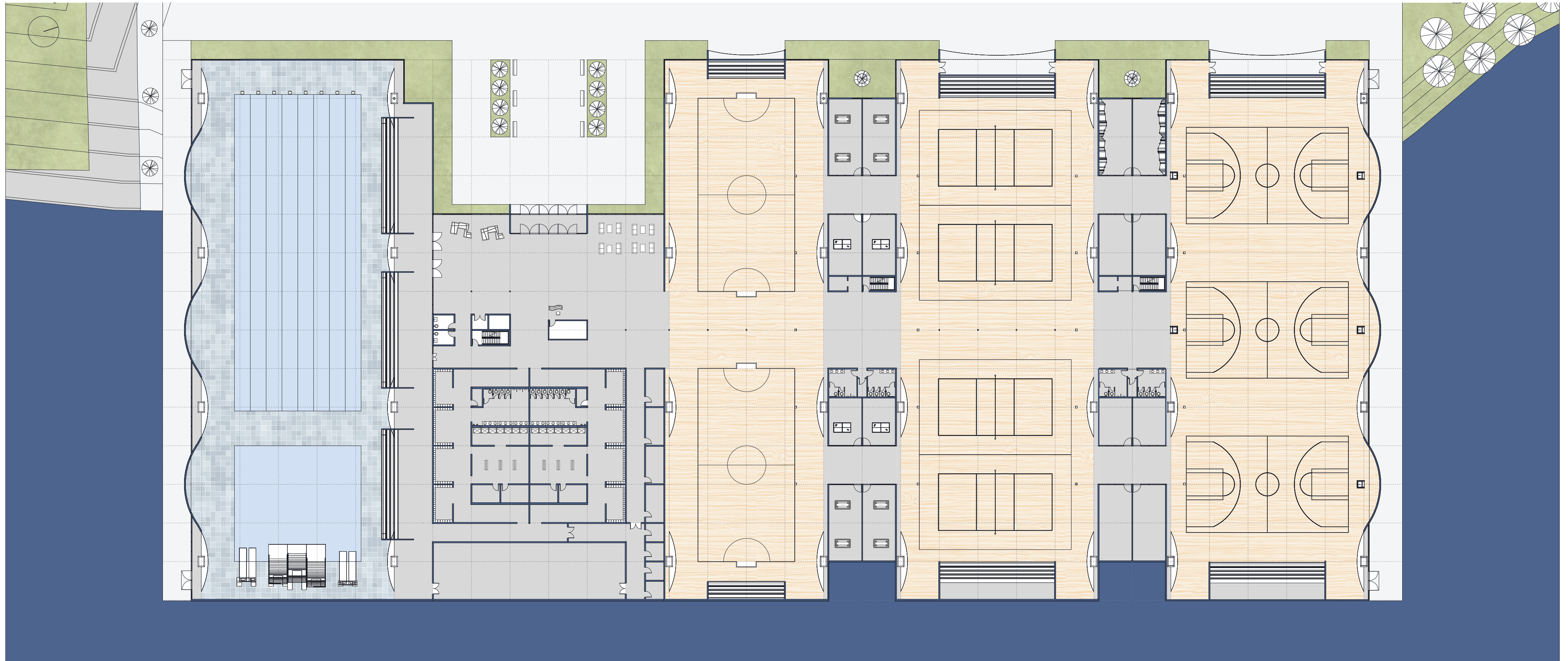
Level 1 As the user enters from the exterior axis, they enter the lobby and encounter an interior axis that is perpendicular to the former. Along this axis are the major spaces within the building, which are the aquatic center, indoor soccer courts, volleyball courts, and basketball courts. If visitors choose to do so, they may keep walking straight along the main entrance axis which will lead them directly to the locker rooms and service desk should they require preparation and additional information before their procession through the building.
