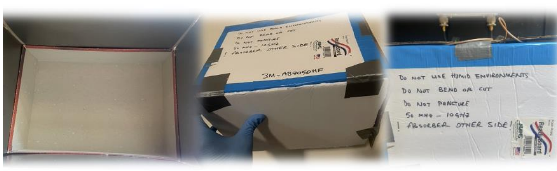
Figure 20: All RF Absorber covered box
