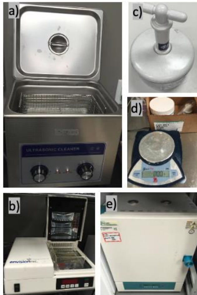
Figure 64: Devices are used for cleaning and curing processes a) Ultrasonic Cleaner b) Optical Curing Flashing Machine c) Hand Vacuum d) Scale e) Oven
