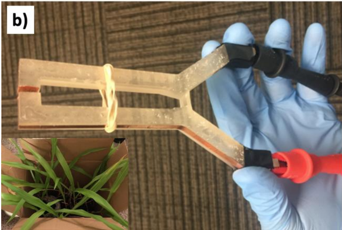
Figure 35: Printed handheld probes for precise measurement
