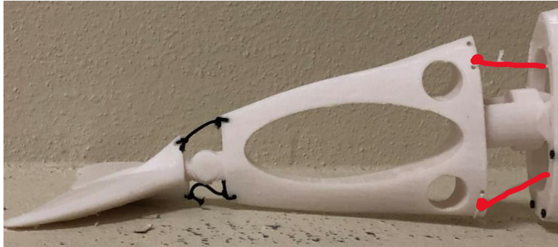
Figure 4.5. (a) Complex tail with 4 joints. (b) Simple tail with 2 joints.
