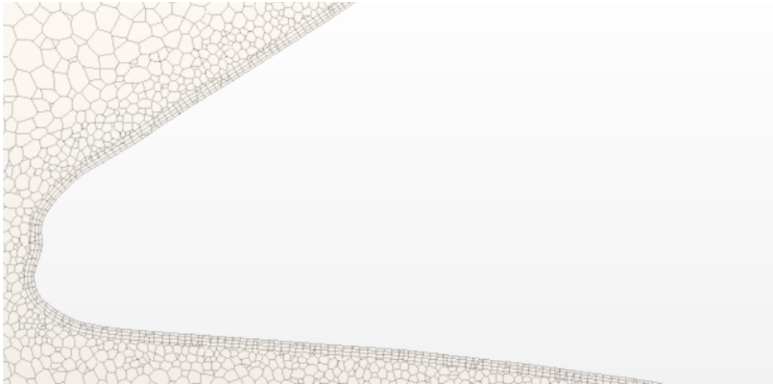
Figure 6.8. Boundary layer prism mesh as seen at rostrum.
