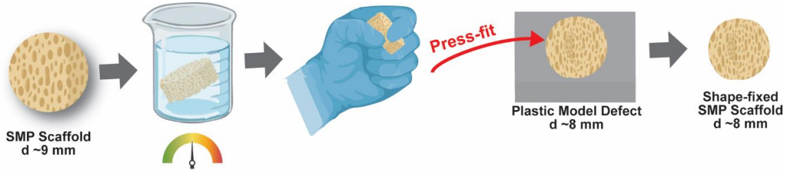
Figure 3-1. Fabricated scaffolds were warmed in saline ( T \sim 55\text{ }^{\circ}\text{C} , 30s) and were press-fitted into a plastic model defect. They were then held at RT for 2 min prior to removal from the model defect to allow for shape fixity. The resulting shape-fixed scaffold discs were used for material characterization and cell studies performed herein.
