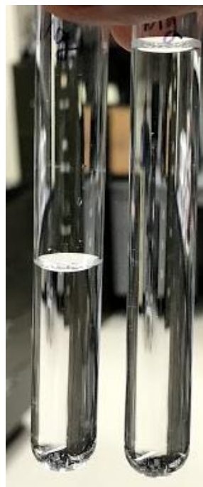
Figure 3-12 Precipitates of 2 mL carbonate/bicarbonate simulant after adding 2 or 6 mL of 0.1 M (a) CaCl 2 and (b) MgCl 2
