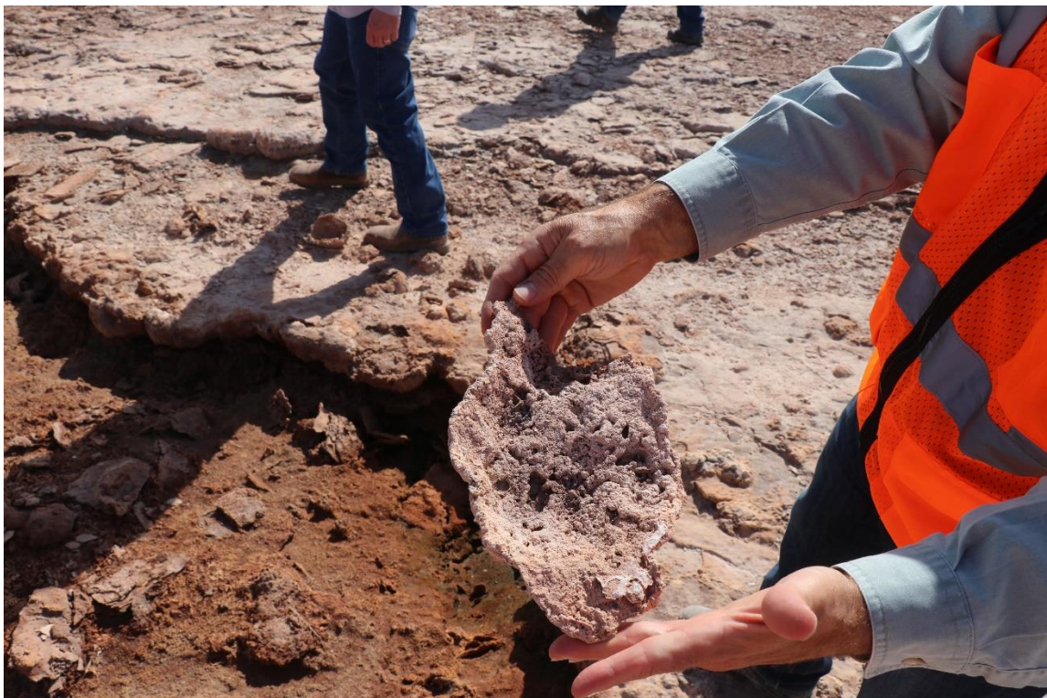
Figure 3-8 Surface crust formed on the top of land area
